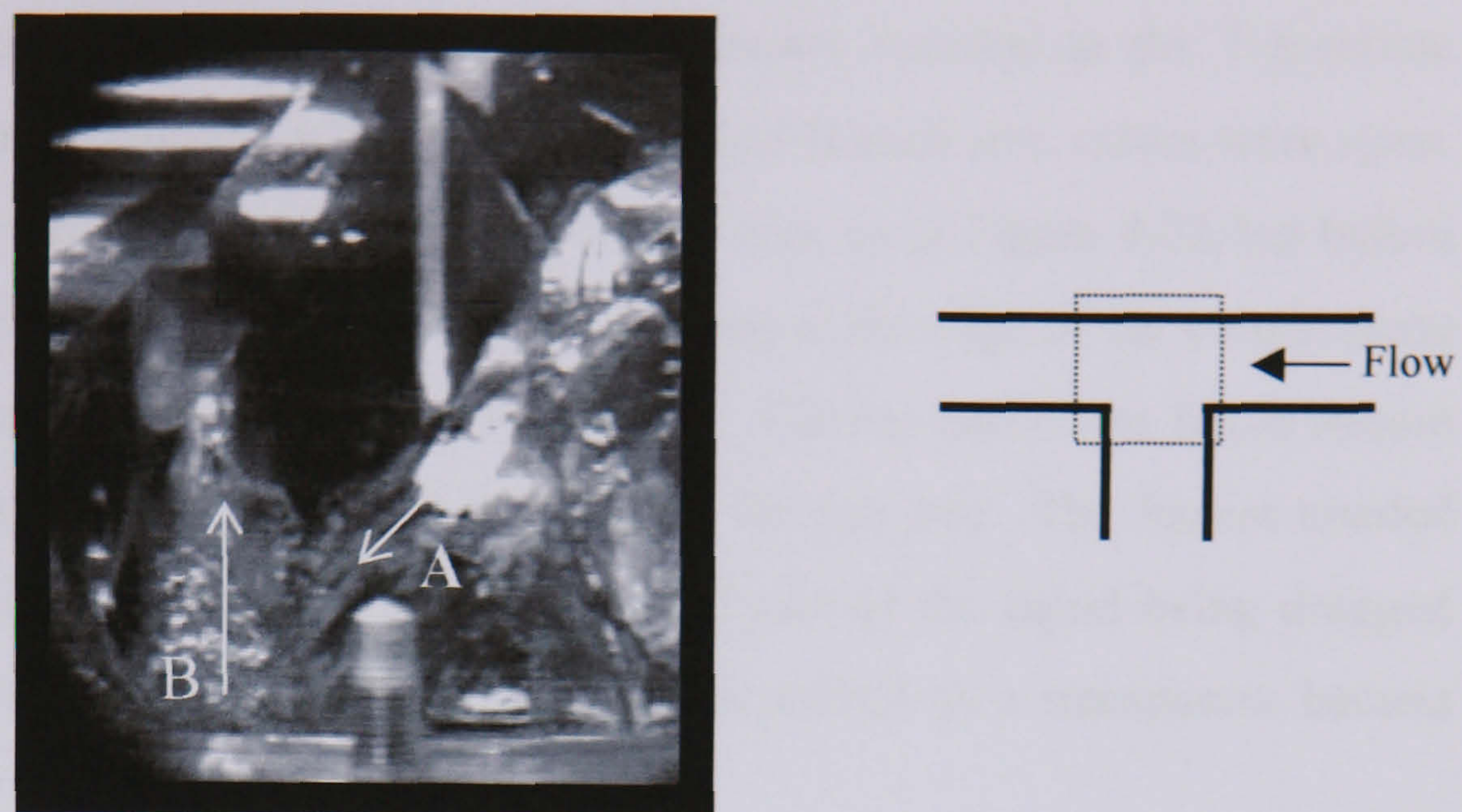
Figure 4-22: Stratified flow (low gas-liquid interface) at the regular T-junction
