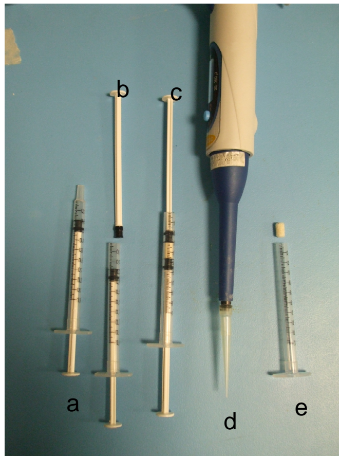
Figure 2-5 The staged process of in situ scaffold production with (a) 1 mL syringe from which the nozzle was removed (b): a secondary plunger was provided and used in (c) to compress particulates before introducing (d) the cell suspension dose. After sintering in the upright position the cell seeded scaffold (e) was ejected.
