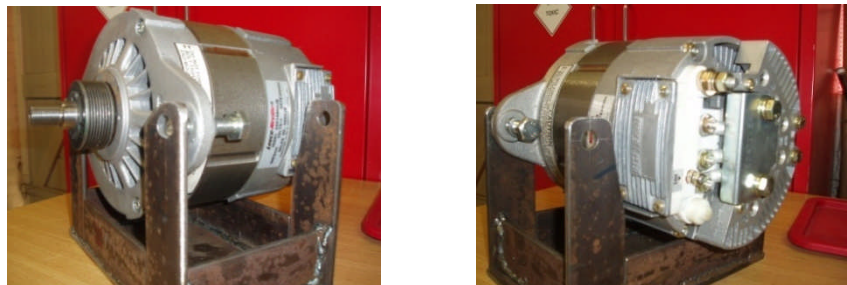
Figure 8.1: End and front view of heavy duty Prestolite alternator
