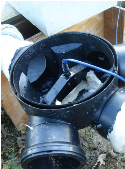
Figure 3.3 Partech IR100C turbidity probe mounted in outflow pipe from the field drain system beneath the Bowl (a); and changes in response through time of sensors mounted in the surface (b) and drain (c) outflow pipes.
