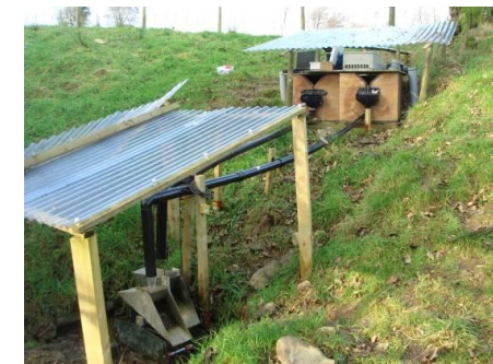
Figure 3.2 (a) Layout of hydrometeorological equipment and supporting infrastructure at experimental pasture on Tyn-y-bryn farm; (b) overland flow trap (beneath wooden boards along downslope edge of the Bowl); (c) box weir/tipping bucket runoff monitoring system. Aerial photography provided by University of Wales Aberystwyth.
