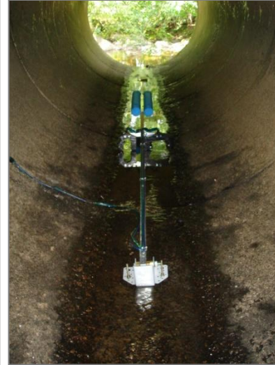
Figure 6.1 (a) Turbidity monitoring equipment, deployed in a culvert at (b) Sheepfold on the Nant Pen-y-cwm and (c) beneath Hirrhos Bridge on the Nant Melin-y-grûg.
