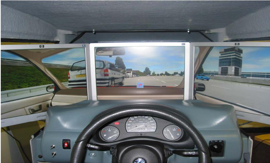
**Figure 5.1. Inside view of the driving simulator**
