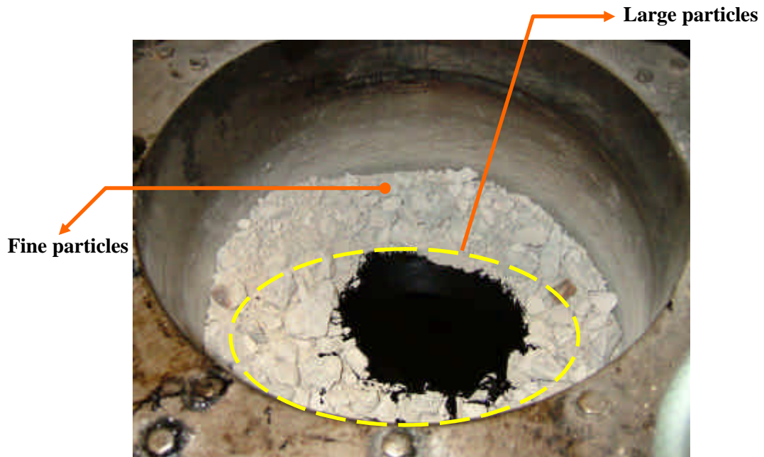
Picture 3.6: Aggregate segregation during dry mixing process
