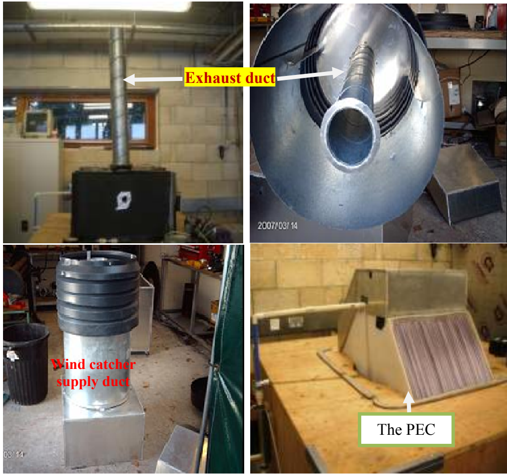
Figure 5.10 Rig fabrication stages
