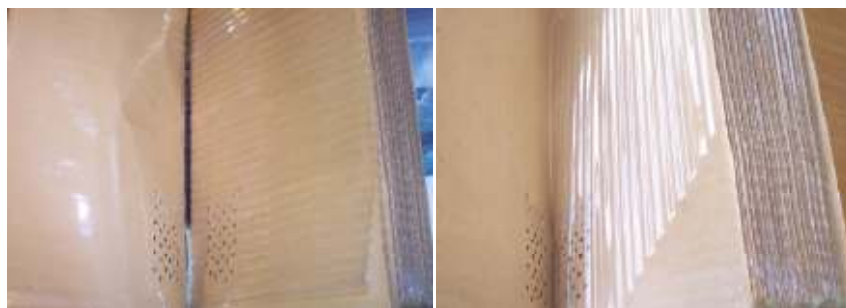
Figure 4.2 Structure of a PEC showing the Wet (Exhaust air) and the dry (Supply air) channels.
