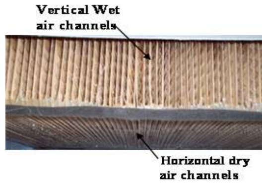
Figure 4.2 Structure of a PEC showing the Wet (Exhaust air) and the dry (Supply air) channels.
