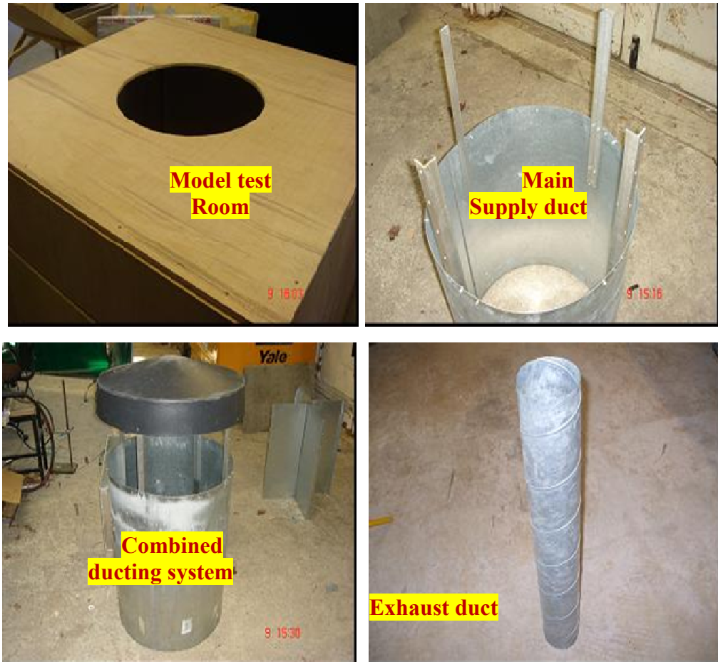
Figure 5.9 Photo showing stages of construction of the test model
