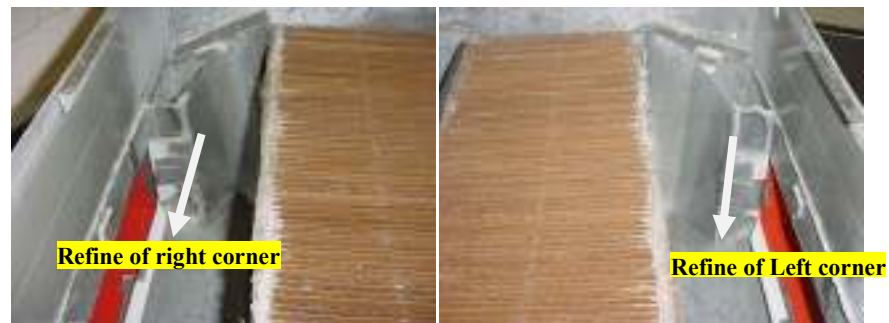
Figure 4.15 Photos showing adjustment to the outlet corners
