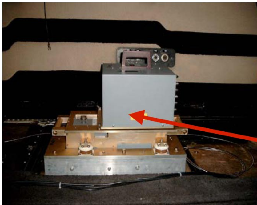
Figure 56 The integrated ALTM sensor with the Applanix DSS camera (adapted from ALTM brochure, 2008)
