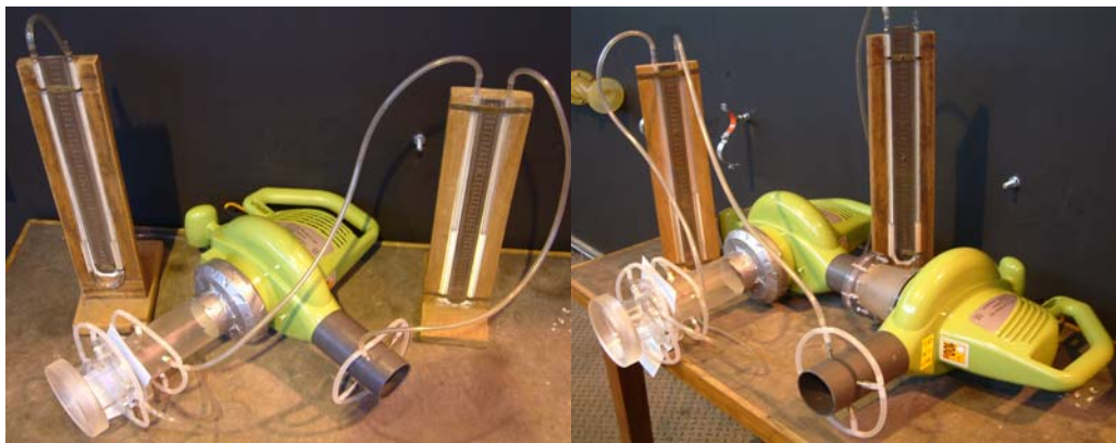
Figure 5.26: Experimental setup for fan tests
