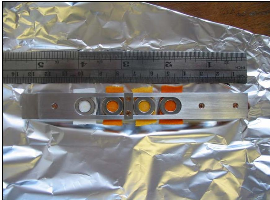
**Figure 2.11** Displays the series of undyed and dyed cloths (from left to right – undyed, 4%, 1% and 9% w/v dyed cloths) clamped into position prior to analysis by XPS.
