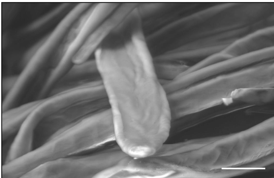
**Figure 4.4** ESEM image of greige fibre at 1000x magnification and spot size 4 $\mu$ m, with scale bar 20 $\mu$ m; displaying natural fibre end in a characteristic tapered shape.
