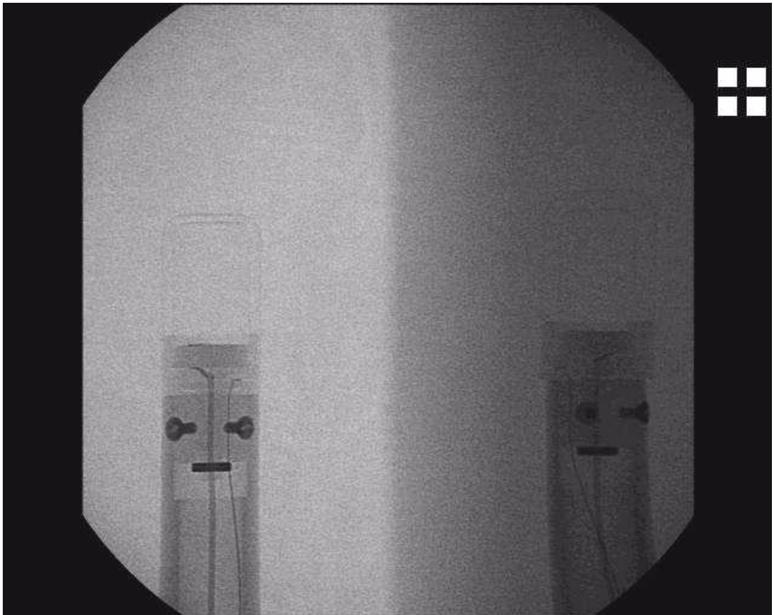
Figure 4.3: Dose meter positions for wedge filter measurements.
