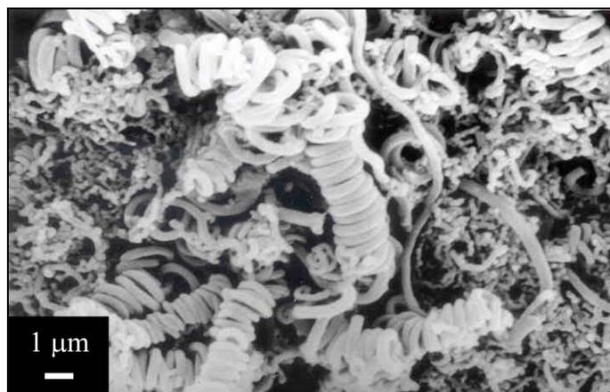
**Figure 7-6** SEM images of CNF catalyst  $\text{Cu}_5\text{Fe}_{85}\text{Ni}_{10}\text{i}$  grown in a quartz reaction vessel
