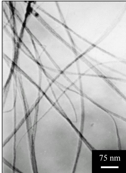
**Figure 2-13** Typical TEM of CNF with smaller diameter grown by the floating catalyst method (Fan *et al.*, 2000)
