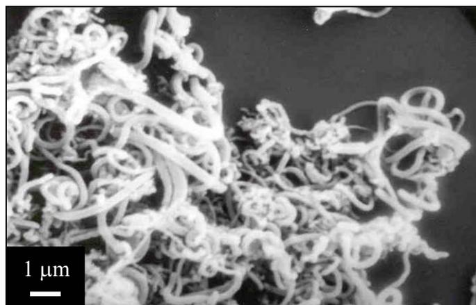
**Figure 7-2** SEM image of CNF grown from pure ethylene using catalyst  $\text{Cu}_5\text{Fe}_{85}\text{Ni}_{10}\text{c}$
