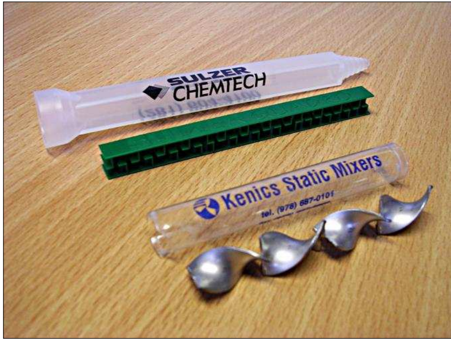
Figure 1.5: Two static mixing devices. Shown at top is a Sulzer Chemtech mixer, with its square cross-section insert. At bottom is a twisted insert from a miniature Kenics static mixer, that causes stretching and folding of the fluid as it is pumped along the pipe.
