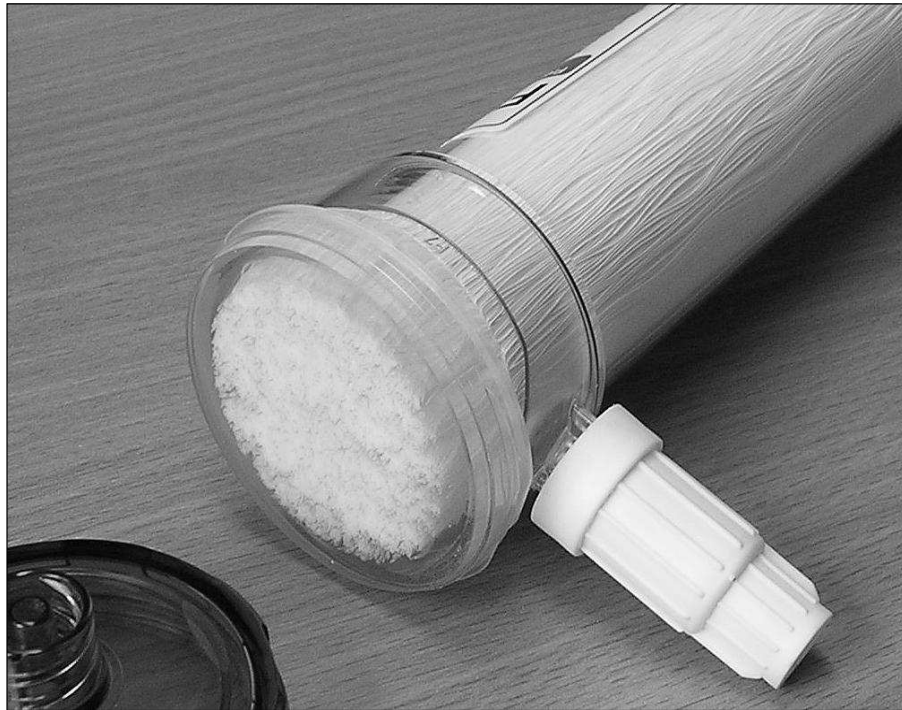
Figure 1.1: An artificial kidney fibre bundle, containing thousands of hollow membrane fibres. Blood is passed along these fibres, whilst another fluid, the dialysate, is passed outside the fibres. Solutes and water are transported across millions of microscopic pores in the fibre walls.
