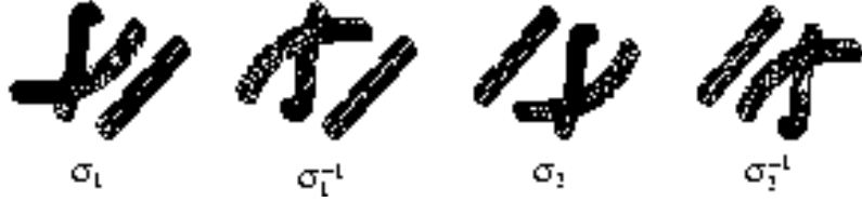
Figure 5.7: Illustrations of the four BPM component units \sigma_1 , \sigma_1^{-1} , \sigma_2 and \sigma_2^{-1} , showing the twisting of the inner pipes. The outer pipe surrounding all the inner pipes is not shown.
