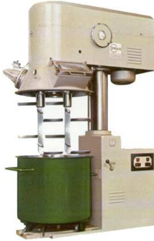
Figure 1.3: A typical industrial planetary mixer. Fluid in a vat is mixed by one or more bladed impellers that rotate as they are moved around.
