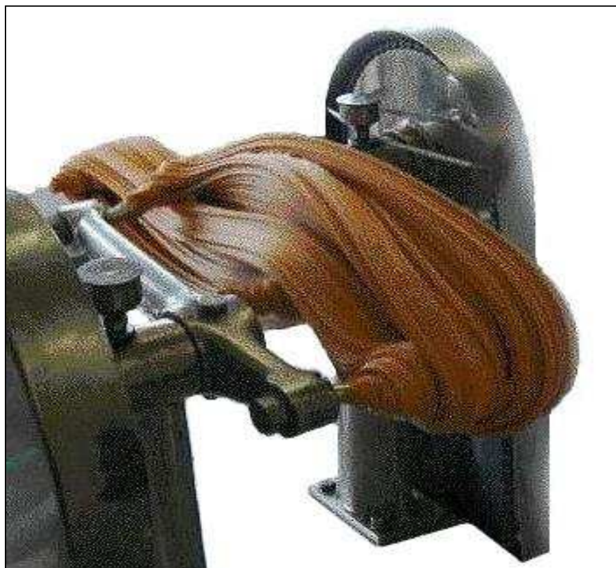
Figure 1.4: A taffy pulling machine, consisting of two motorised arms, each with two protruding taffy covered rods. The arms rotate so that the prong trajectories intersect causing rapid stretching of the taffy, and folding of air into the mixture.
