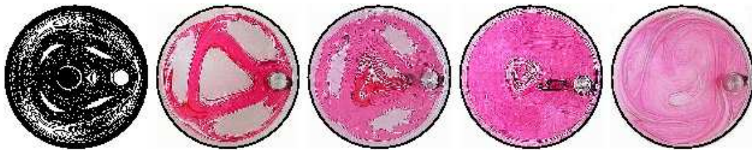
Figure 3.12: From left to right: iterated mapping plot, showing islands in numerical simulation of Stokes flow; large time dye-advection experiments in glycerol, with Re = 0.1, 1, 3, 10 .
