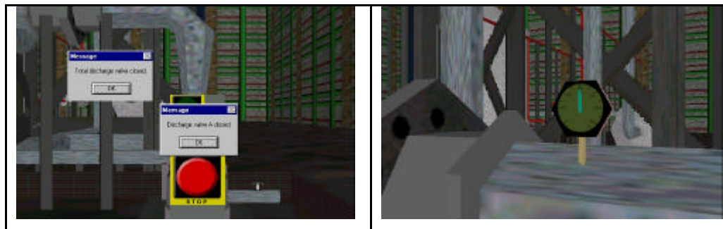
Figure 4.18: Message boxes from the pump training system – The pressure meter indicates that the discharge line is pressurised.
