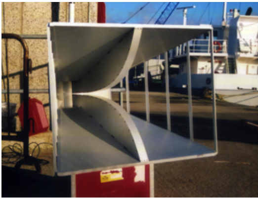
Figure 5.9: Wide-bandpass Horn antenna on quayside in front of tide gauge building in Aberdeen Harbour
