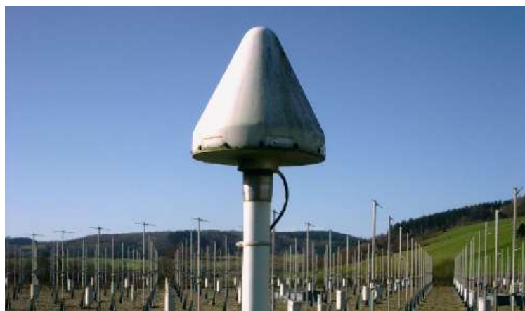
Figure 5.14: GPS antenna at ABYW with antenna array of the NERC MST radar profiler in the background (Courtesy of the Met Office)
