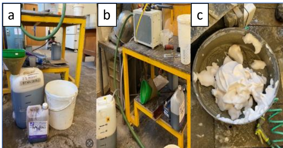
Figure 3.2: Foam producing: (a). Foaming agent (b). Foam machine (c). Foam
