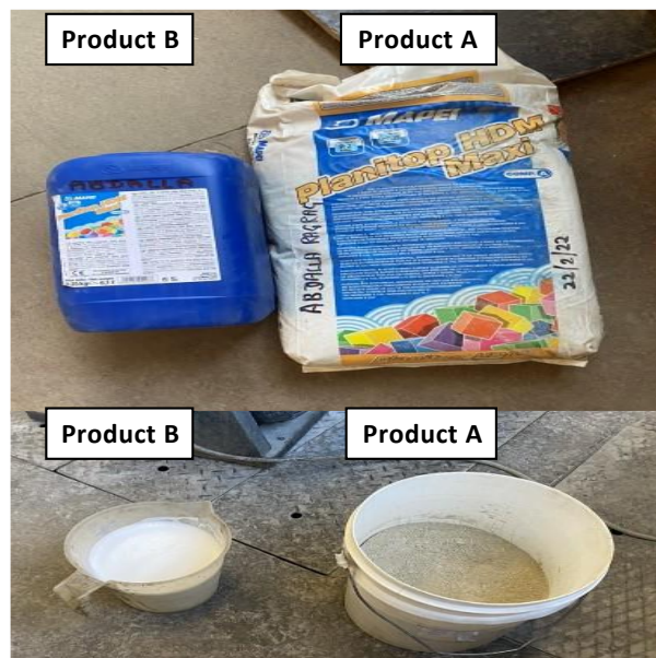
Figure 5.2: Ready mix (Planitop HDM Maxi) - Component A and Component B
