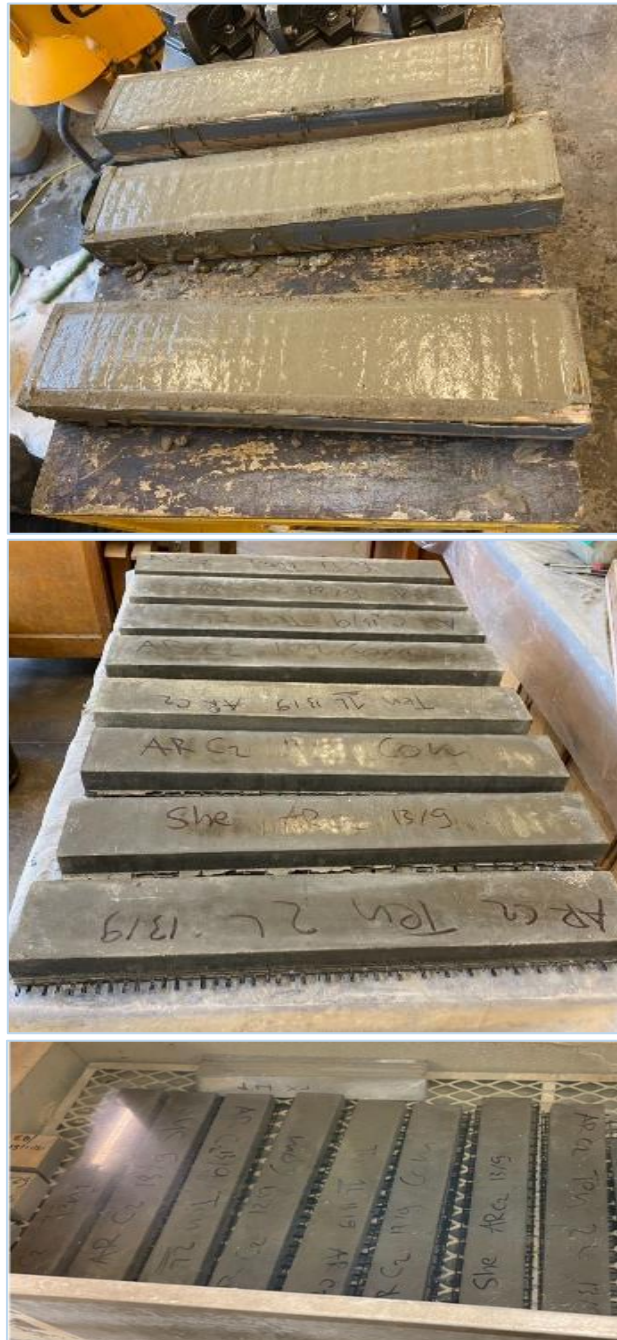
Figure 5.7: Samples casting and curing.
