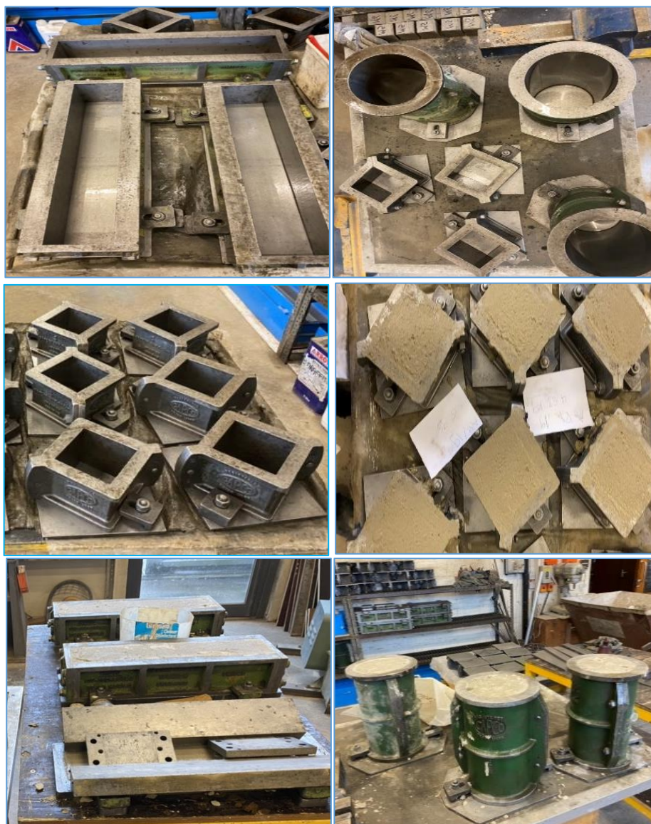
Figure 3.6: Prepare and apply release oil on the specimen, then position the foamed concrete mix.
