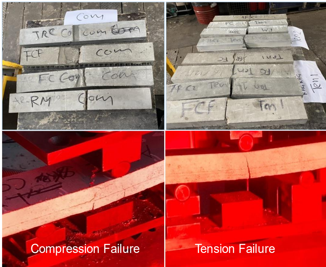
Figure 5.15: Comparison between compression failure and tension failure.
