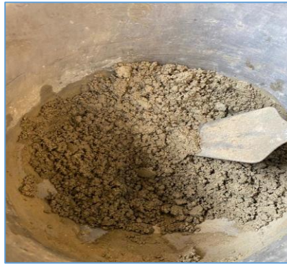
Figure 3.13: Excluded non-integrated mix (FC-7 mix)
