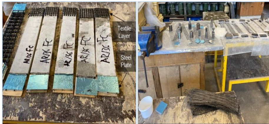
Figure 5.20: Steel plates securely anchored and reinforced with additional textile layers at the other end of the samples
