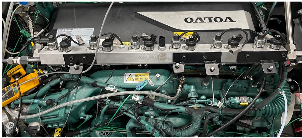
Figure 6.8: New integrated NH_3 and H_2 rail.
