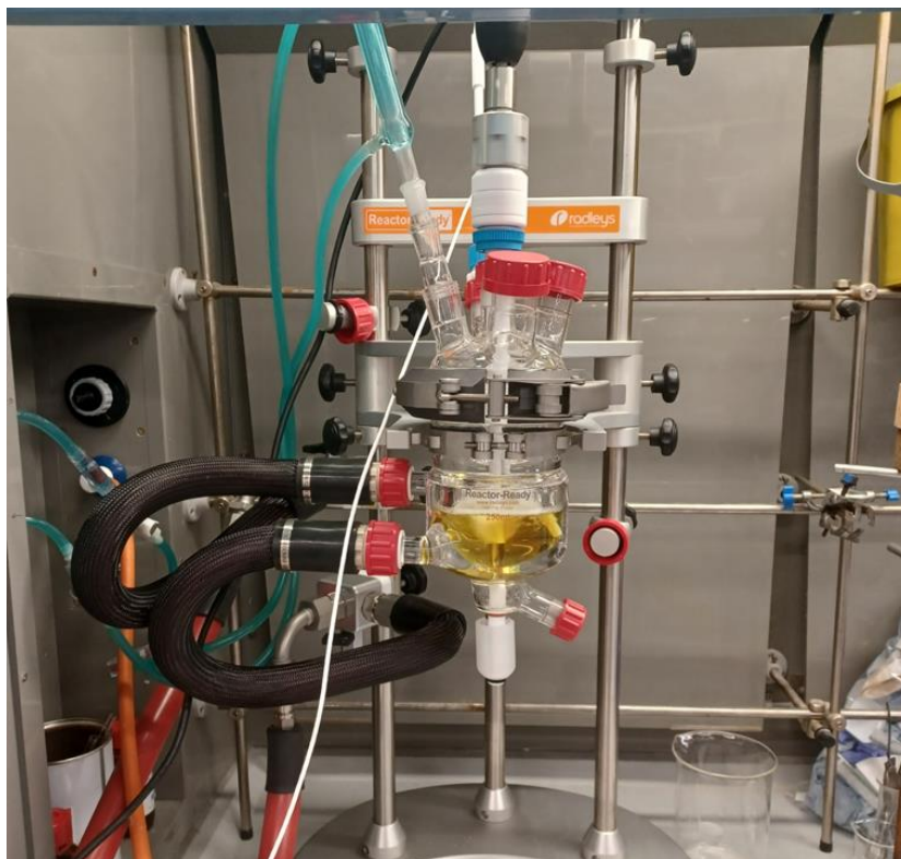
Figure 28: large scale reaction in a jacketed vessel
