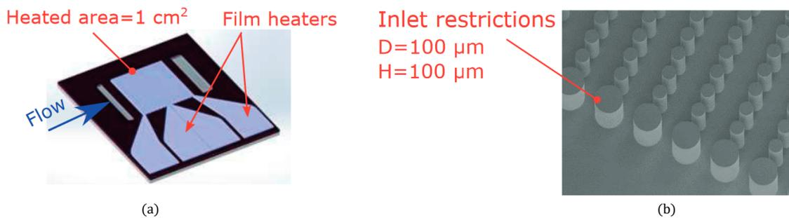
Figure 6.1: (a) Micro-pin fin evaporator bottom side with aluminium film heaters. (b) Inlet restrictions before the micro-pin fin array, from Falsetti et al. [42].
