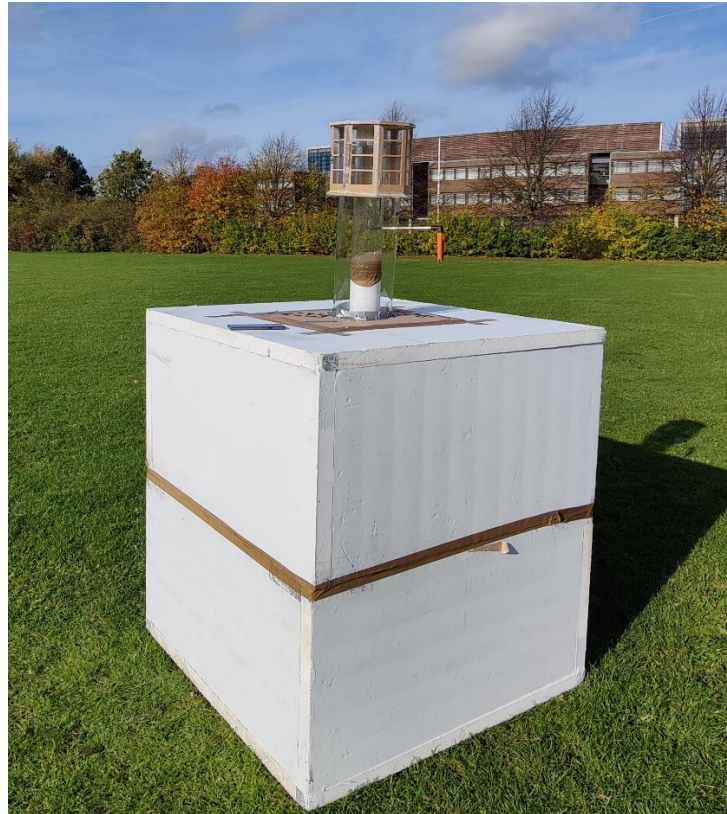
Figure 3.23 Field test model photo of flap fin inlet windcatcher
