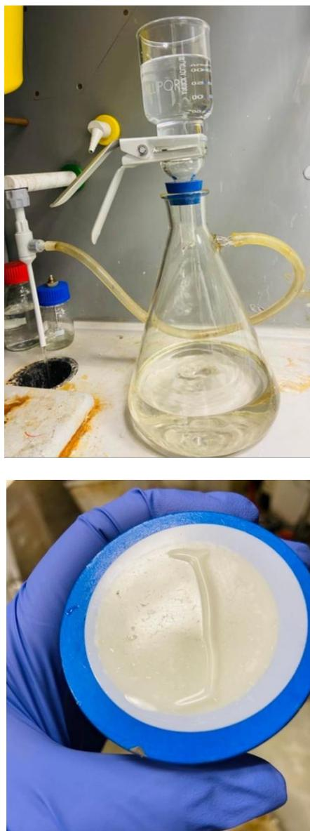
*Figure 26. The image at the top shows the vacuum system used for DMF filtration before the printing process, and the one at the bottom shows an example of the impurities detected by the filter.*
