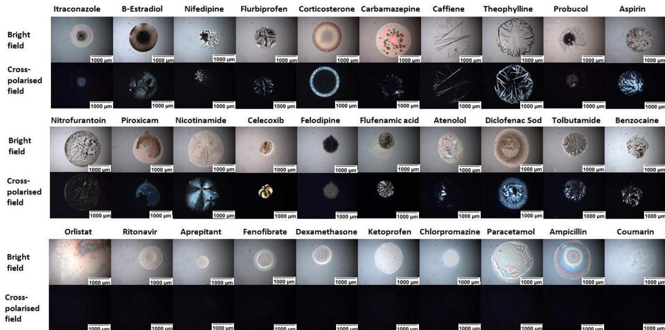
Figure 52. The figure shows different APIs recrystallisation profiles used in this study (final mass 1000-1100 ng) printed using 2D piezoelectric inkjet printer. All images are reported without (top row) and with (bottom row of each set) cross-polarised filters. Images of all APIs are depicted six months from solvent evaporation while storage in accelerated conditions (75% relative humidity and 40°C in stability oven).
