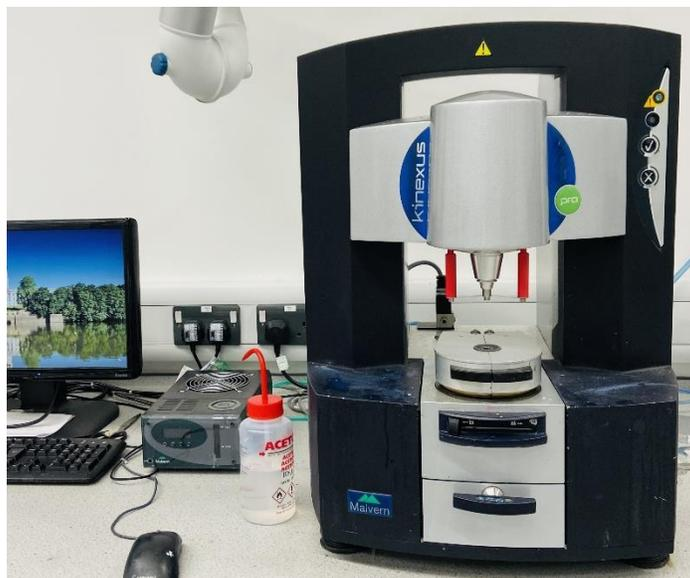
*Figure 34. Malvern Instruments Kinexus Pro Research Rheometer used to measure the viscosity of the ink.*
