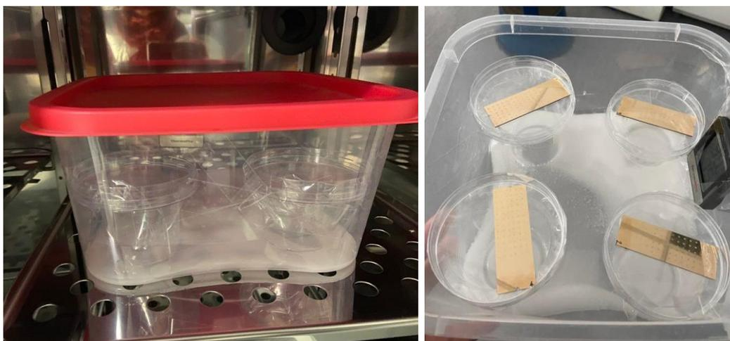
*Figure 31. Microarray storage at 75% RH  $\pm$  5% at 40°C in a stability oven. as an accelerated condition for the stability study.*
