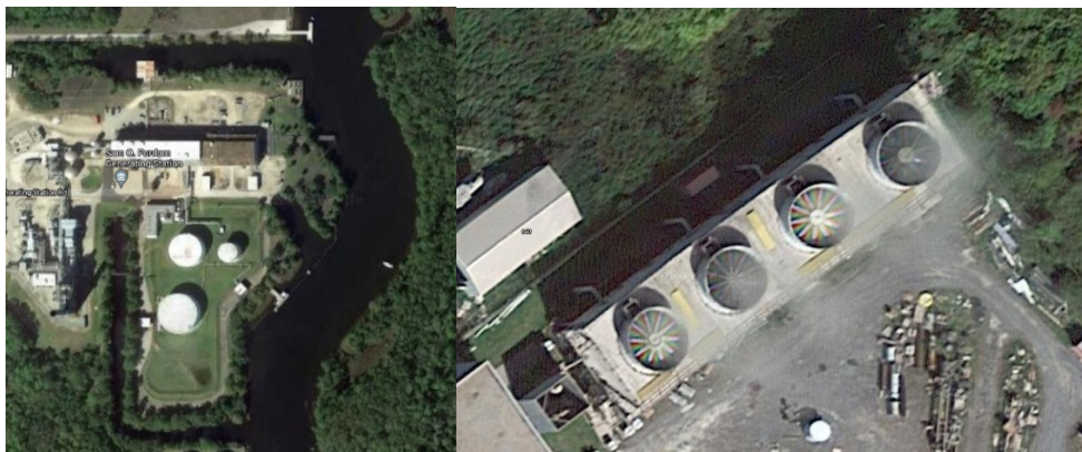
Figure 3.3. A once-through cooling system ( left ) and cooling towers in operation ( right ) identified via satellite image on Google Earth.
