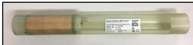
Figure 3.6. ^{23}\text{Na} probe by Bruker with an internal diameter of 25 mm used for sodium experiments.
