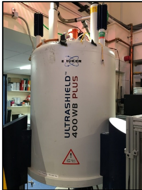
Figure 3.5. Ultra-high field 9.4 T NMR spectrometer by Bruker. Temperature inside the bore can be controlled by the temperature control unit.
