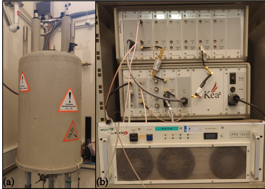
Figure 4.4. (a) The 9.4T poor-shielded NMR magnet Oxford and (b) a portable high-frequency spectrometer Kea 2 with an external amplifier LPPA 14020.
