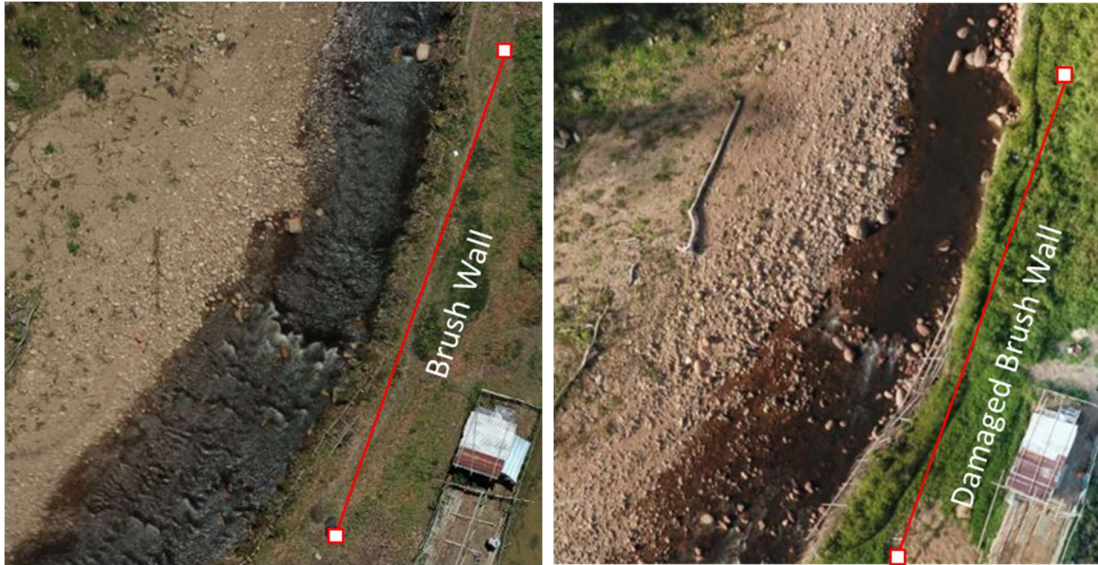
Plate 4.3: Cropped section of Site A, captured in June 2019 (left) and February 2020 (right).
