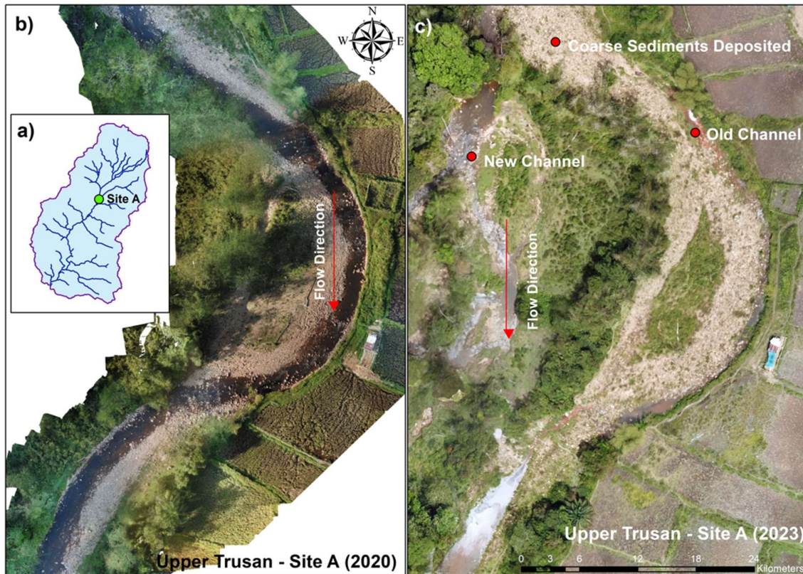
Figure 7.1: a) Location of Site A, b) Orthomosaic of Site A surveyed in 2020 and c) 2023 before and after a large flood.
