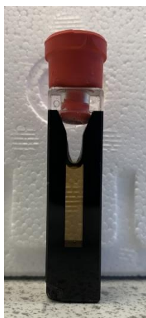
Figure 81 – Quartz cuvette containing the [4Fe-4S] cluster maquette sample sealed under anaerobic conditions.
