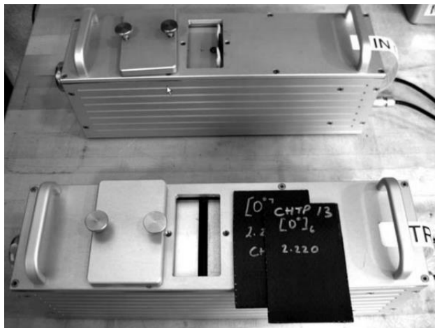
Figure 5-1 Hukseflux devices: THASYS (front) for through-thickness measurement and THISYS for in-plane measurement (back) [148]
