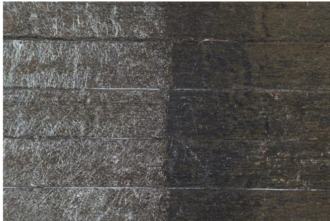
Figure 3-11 Macro-photograph of binder surfaces of processed and peeled static samples at the boundary region between precrack area (right) and peeling area (left) (Veils left on the binder surfaces are shown on the left-hand side. Peeling direction is from right to left.)
