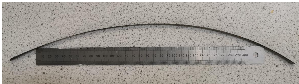
Figure 5-11 Tape with residual deformation after cutting from bobbin termed 'bent' tape (Top surface is veil surface and bottom surface is binder surface.)
