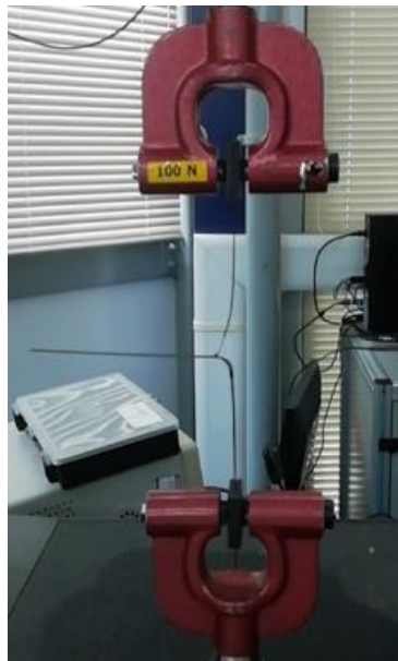
Figure 3-6 Experimental setup for T-peel tests
