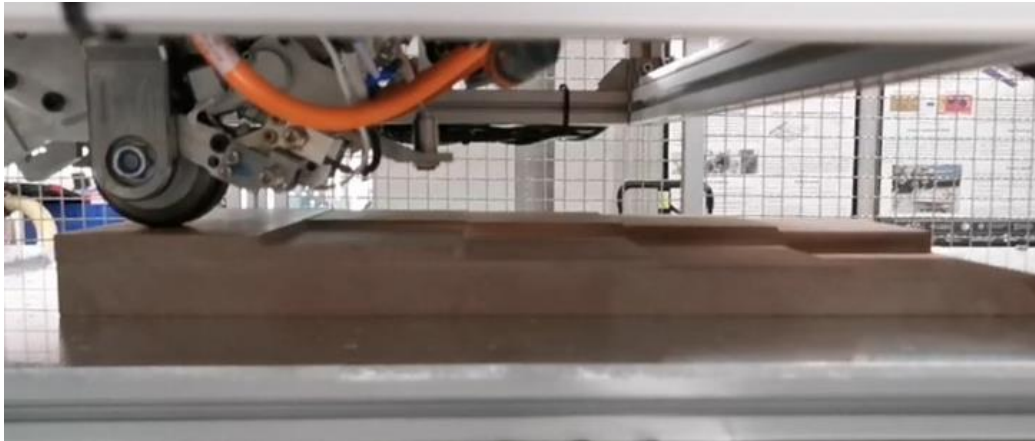
Figure 6-7 ADFP deposition head compaction on a tool with steps
