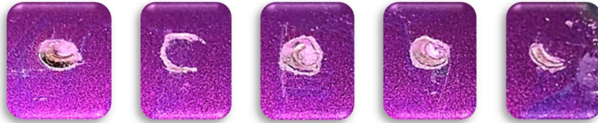
Figure 5.47: Green stumps after tensile testing on treated silicon nitride.
