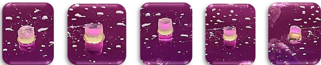
Figure 5.49: Stumps after tensile testing with 8 minutes PBC on treated substrate.
