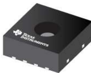
Figure 1.2: Example gas sensor package by Texas Instruments [25]
