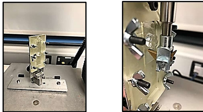
Figure 3.31: Shear test sample secured in TA machine for adhesion testing. [Left] Test bracket clamped on adaptor plate and secured to base plate, [Right] frustum test shear test piece on PC in place for testing.
