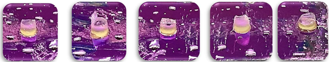
Figure 5.48: Stumps after tensile testing with 2 minutes PBC on treated substrate.
