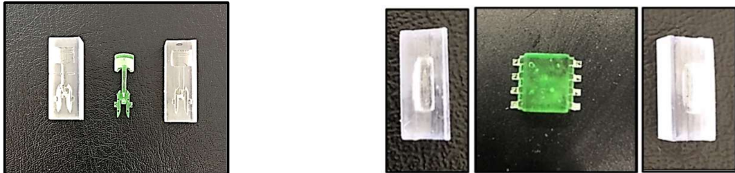
Figure 4.36: Example test geometries with 2-part adaptors. [Left] Example piston and [right] semi-conductor geometry constructed on an Anycubic SLA machine with corresponding 2-part adaptor pieces (constructed on a Form 2 SLA machine).
