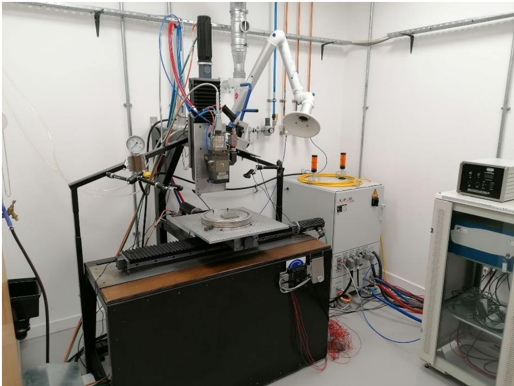
Figure 3.1 Laser cladding system
