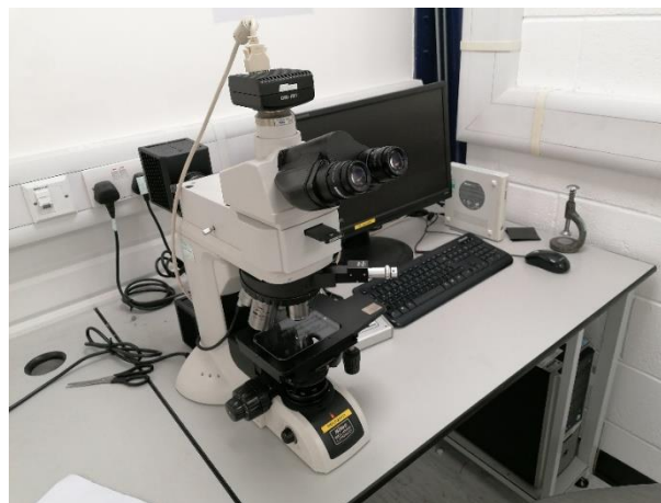
Figure 3.31 Nikon LV100ND optical microscope with Nikon DS-Ri1 camera
