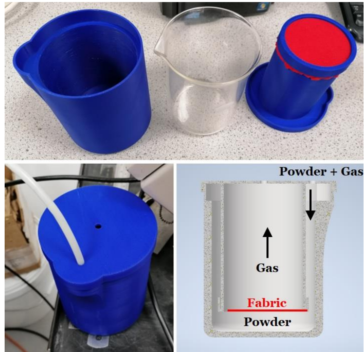
Figure 3.4 Powder collector device
