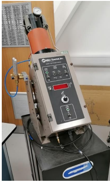
Figure 3.2 Powder delivery system
