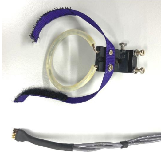
Figure 16. Photographs of the custom-designed harness and 6-way plug connector.
