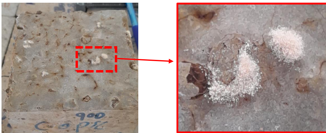
Figure 4.42 White-rot fungi on outer surface of coarse OPSC
