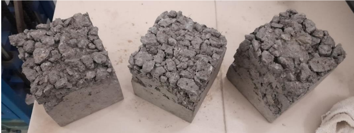
Figure 4.24 Deficiency in cement content at 350 kg/m 3
