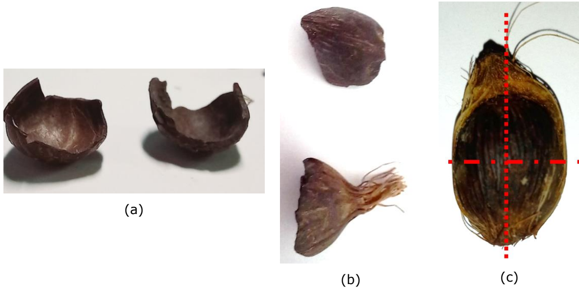
Figure 4.2 (a) Half-hollow-spherical shapes, (b) Common Tenera OPS shapes and (c) Unbroken OPS shell with cracking pattern, horizontal or vertical
