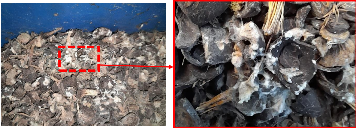
Figure 4.41 Rotting of Tenera OPS left damp for over 6 months
