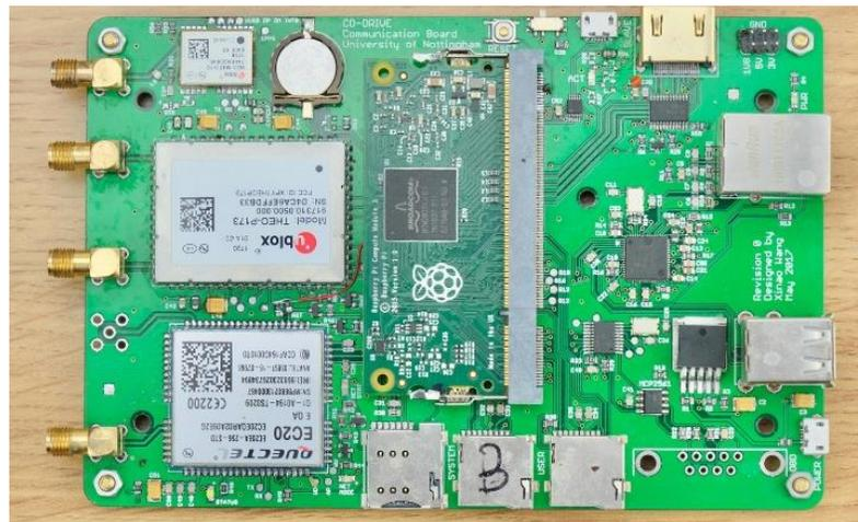
Figure 12: All-in-one OBU assembled PCB.
