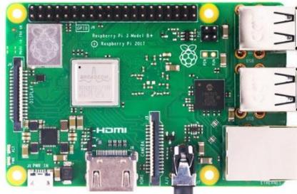
Figure 5: Raspberry Pi 3 Model B+
