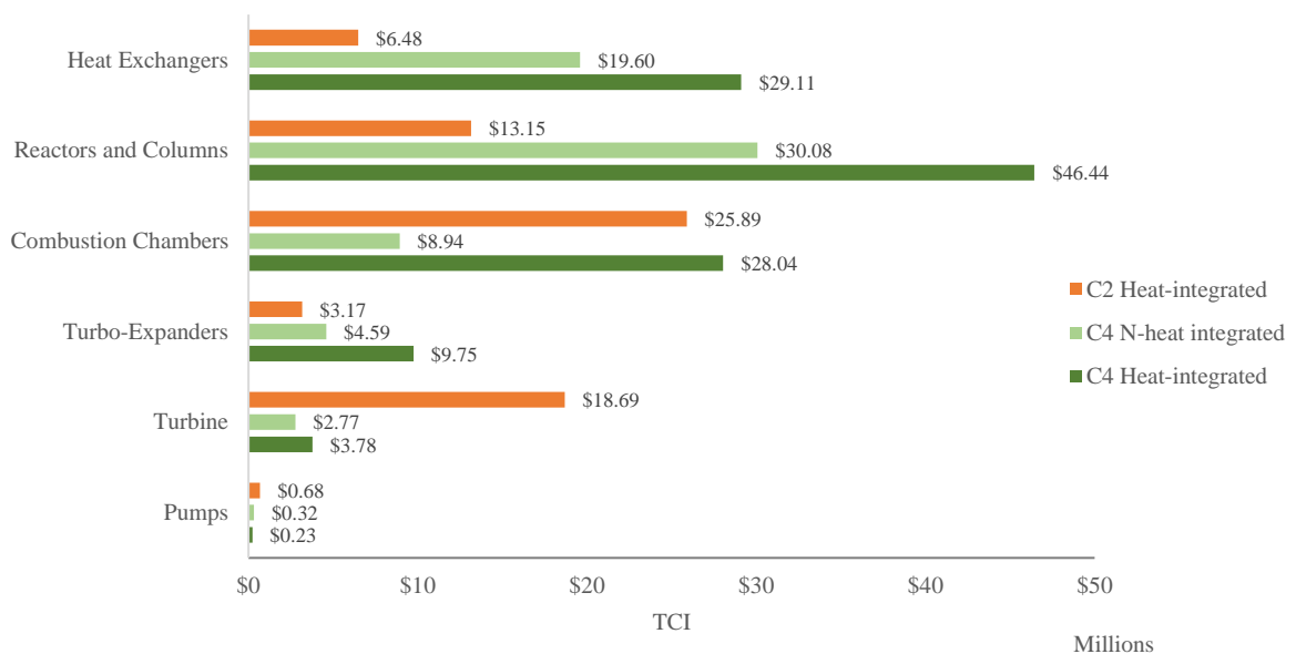
Figure 7.2. Chart showing the breakdown of the TCI of proposed C 2 and both C 4 route-to-SAF plants.
