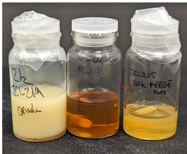
Appendix Figure 31 Samples of pEEGE synthesised using anionic ROP. Left to right: entries 1,2,4 from Table 24. Left sample appears opaque due to precipitated KOH.
