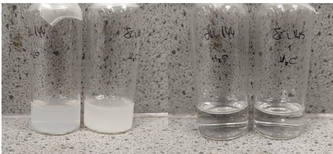
Figure 77 PG4-DMS-2SA (left) and PG4-DMS-3SA (right) undergo rapid dissolution into water as pH is raised.
