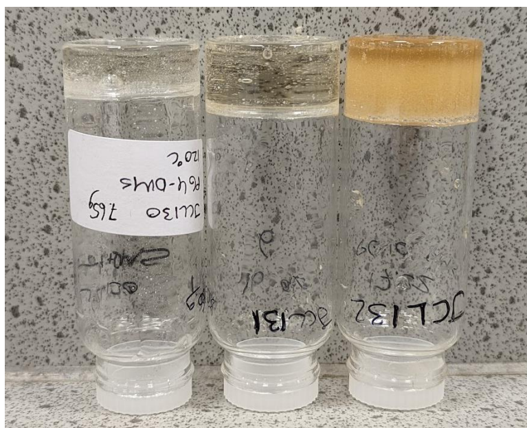
Figure 63 Various lengths of polyglycerol building blocks were polytransesterified with DMS. From left to right: PG4-DMS, PG6-DMS, and PG10-DMS.
