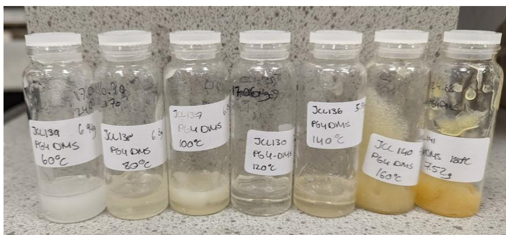
Figure 68 PG4-DMS Synthesised at a variety of temperatures. From left to right: 60, 80, 100, 120, 140, 160, 180 ^\circ\text{C} .
