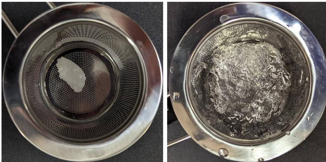
Figure 99 PG4-1.5DMS before (left) and after (right) 24 h submersion in water.
