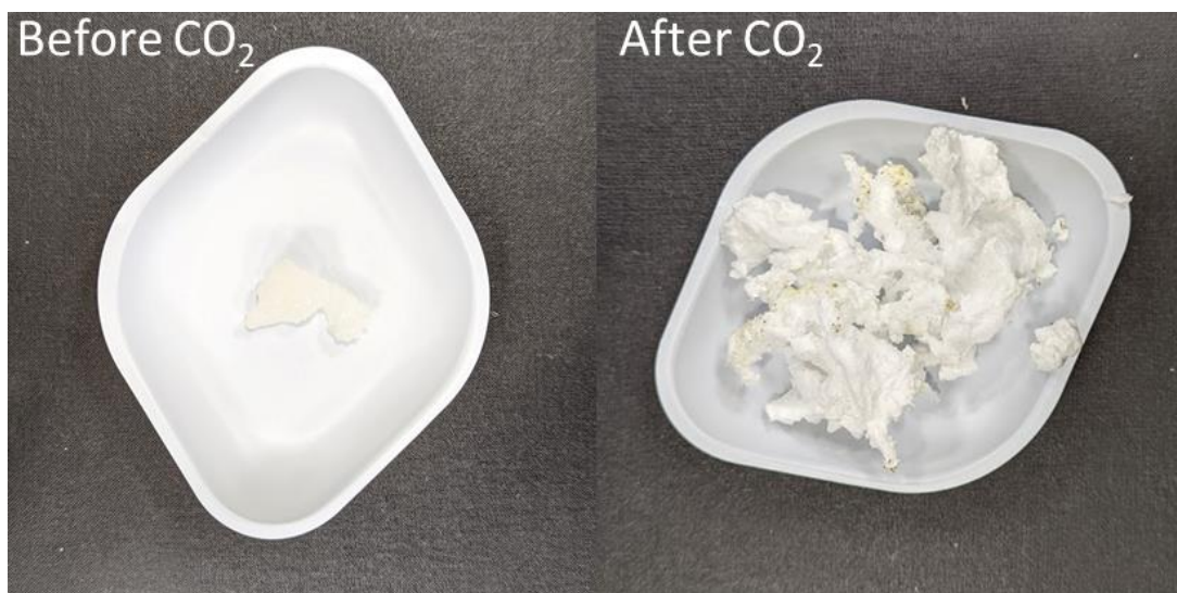
Figure 81 Crosslinked PG4DMS before (left), and after (right) functionalisation with succinic anhydride in scCO_2 . Significant foaming was observed upon depressurisation of the reaction vessel.
