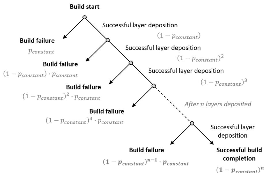
**Figure 2.13: Discrete event probability tree for layer-wise calculation of build failure probability, adapted from Baumers et al. (2017)**
