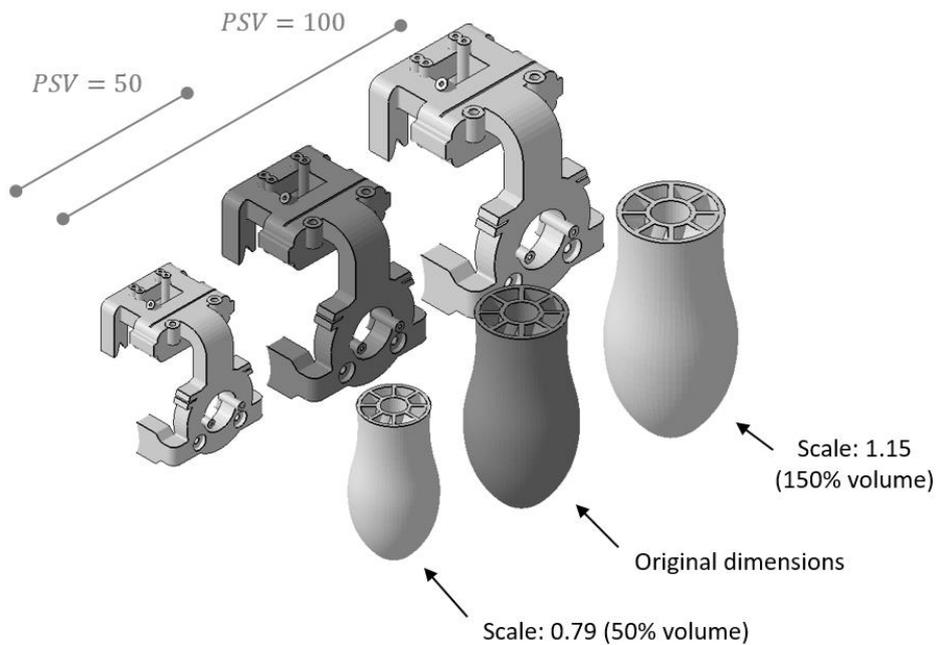
**Figure 3.12: Product variety represented by scaled versions of test parts, with corresponding Part Size Variety (PSV) factor values**
