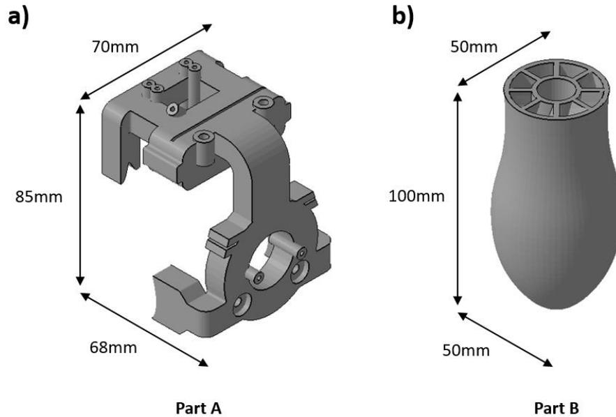
**Figure 3.8: Subset of test parts used for operations approach simulation study**
