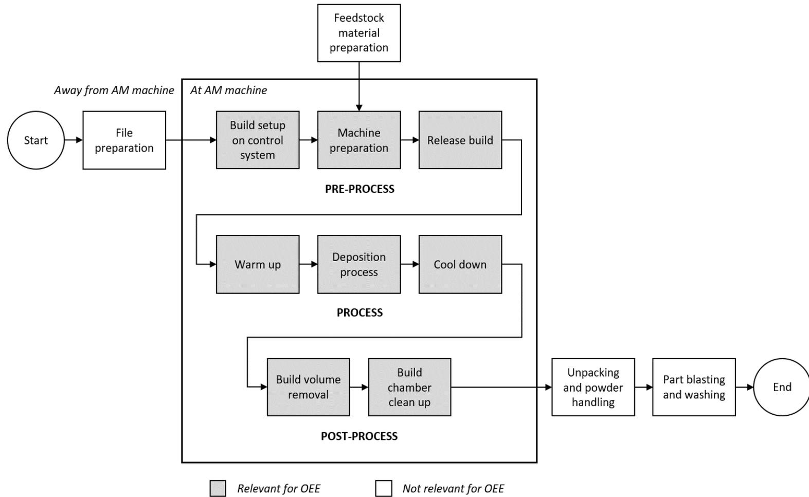
**Figure 3.7: AM process workflow for polymer laser sintering and relevant steps for OEE**
