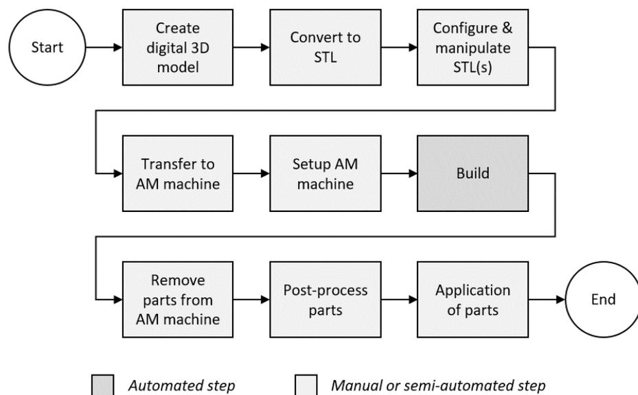
**Figure 2.1: General AM workflow, inspired by Gibson, Rosen and Stucker (2015, p. 5) and Gardan (2016)**
