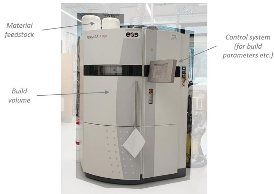
**Figure 2.3: EOS Formiga P100 laser sintering machine in research laboratory**
