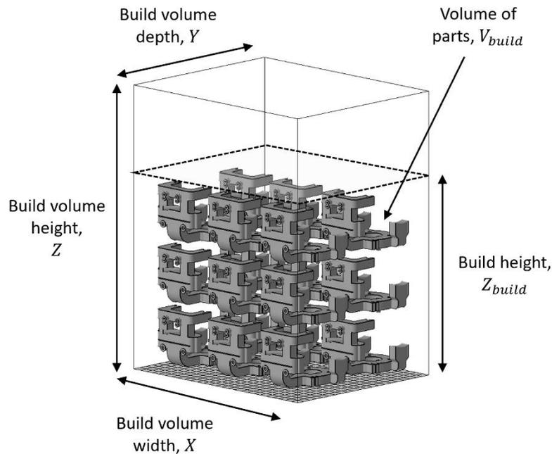
Figure 3.5: Generic build job with key parameters for process metrics
