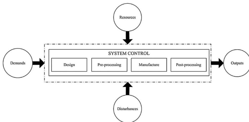
Figure 7.2: Industrial AM system definition, taken from Eysers and Potter (2017)
