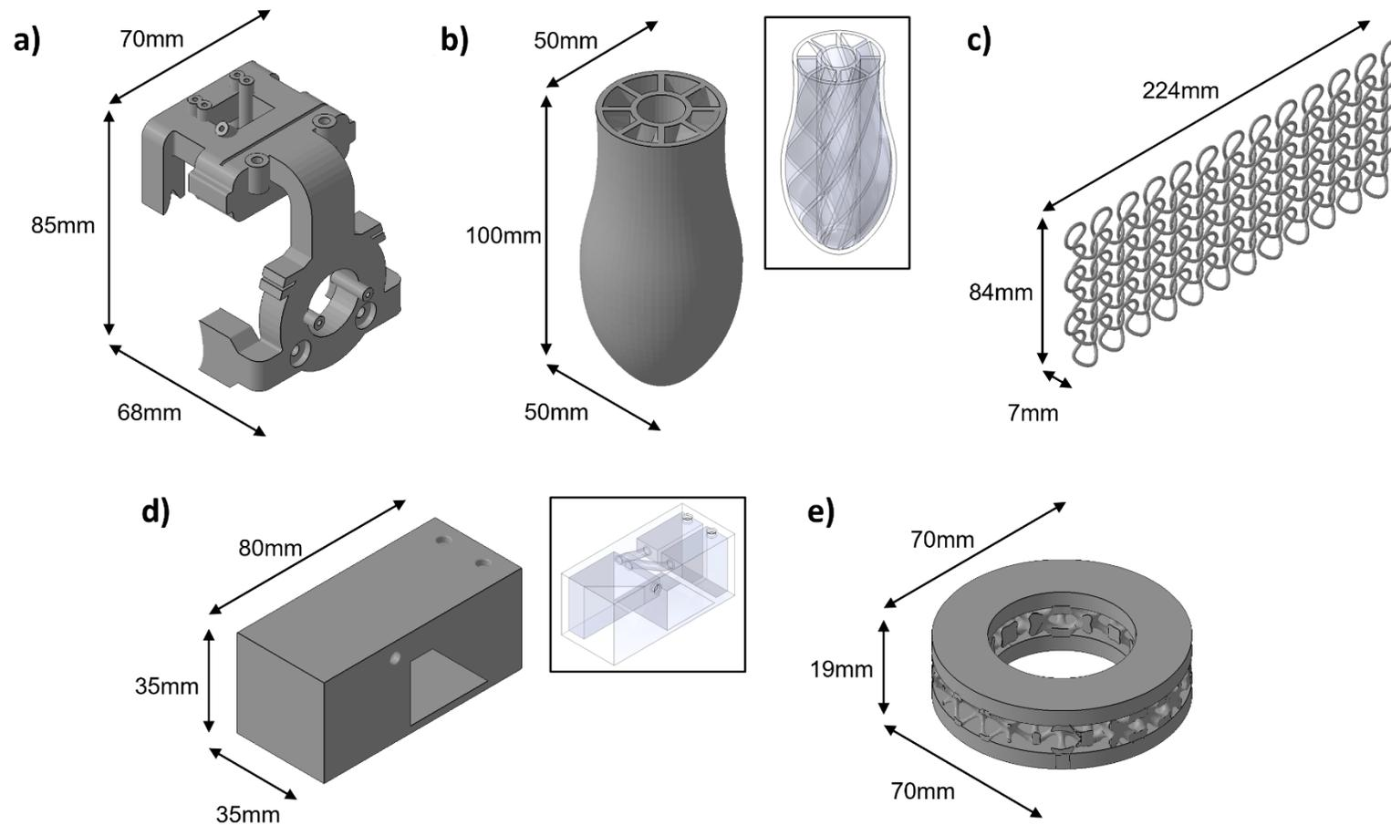
Figure 3.4: Test part designs – a) surgical guide, b) UAV body section, c) chainmail fabric, d) reaction device, and e) mechanical support
