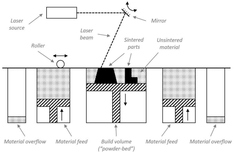
**Figure 2.2: Schematic of the laser sintering process, inspired by Lohfeld and McHugh (2012)**
