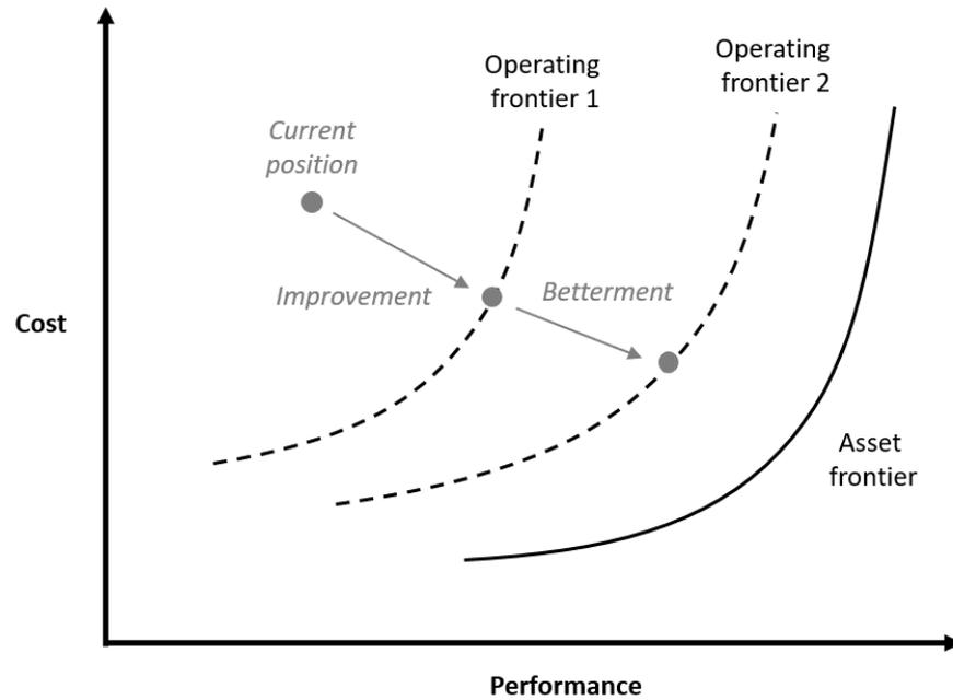
**Figure 1.4: Operating and asset frontiers for manufacturing systems, adapted from Schmenner and Swink (1998)**
