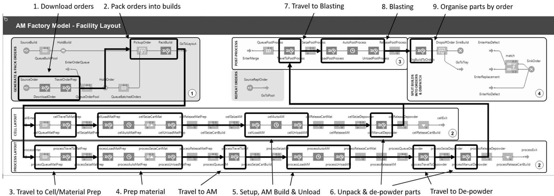
Figure 3.30: Annotated snapshot of facility layout simulation implementation in Anylogic
