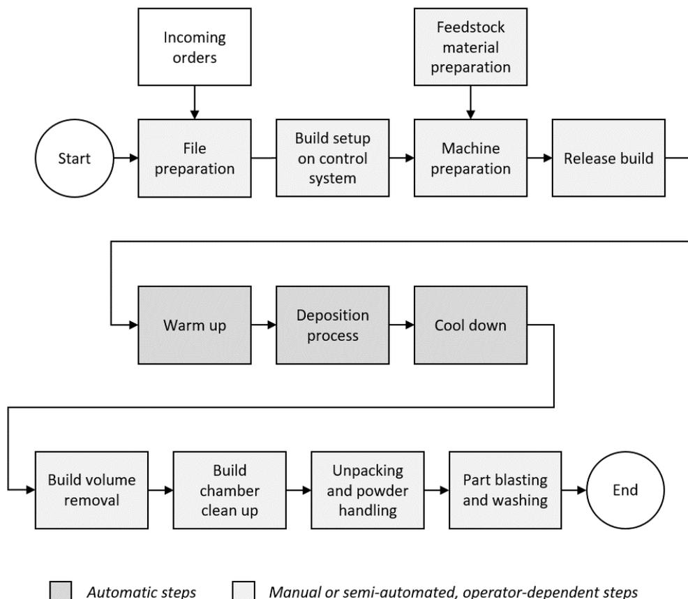
Figure 3.3: Polymer laser sintering workflow for make-to-order production
