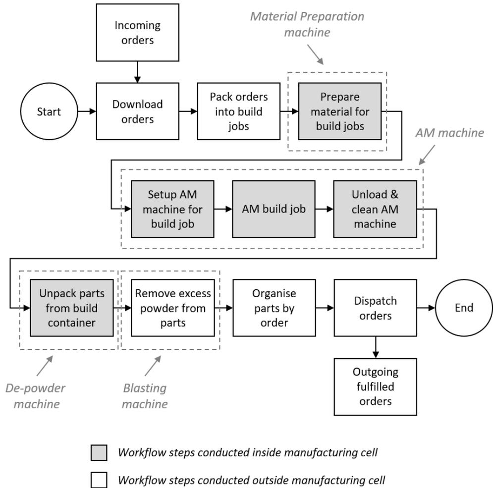
**Figure 3.17: Make-to-order workflow for laser sintering at case study company**
