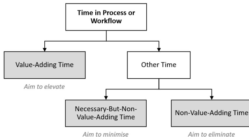
**Figure 2.9: Relationship between time and value creation in a manufacturing workflow**
