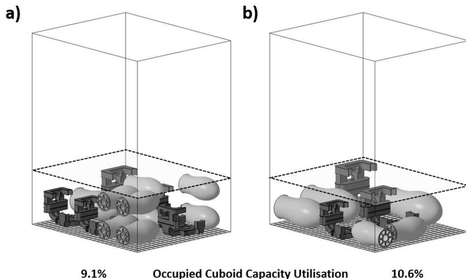
**Figure 4.14: Demonstration of part packing for experiments at a) PSV = 50 and b) PSV = 100, with respective values for occupied cuboid capacity utilisation**
