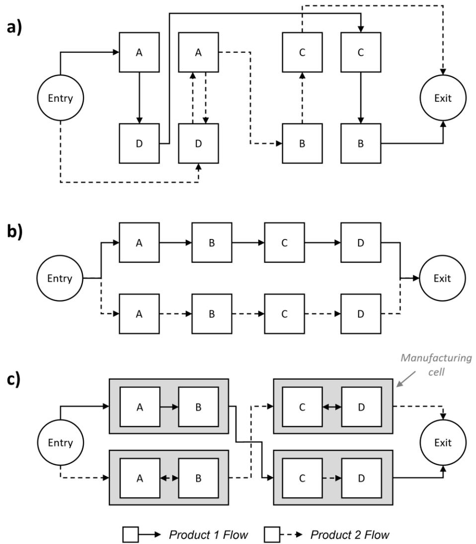
**Figure 2.14: Example flows of different products through facility with a) process layout, b) line layout, and c) cellular layout**
