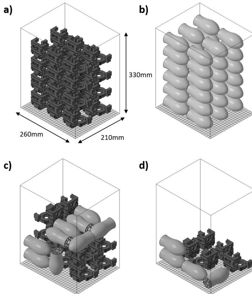
**Figure 4.3: Typical packing of parts in builds for a) IB-MtS part A batches, b) IB-MtS part B batches, c) CM-MtO, and d) LTM-MtO operations approaches**
