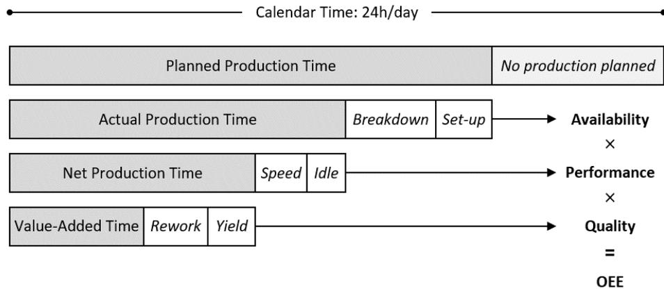
**Figure 2.10: Schematic summary of the six production losses (white boxes), alongside the OEE and its constituent metrics**
