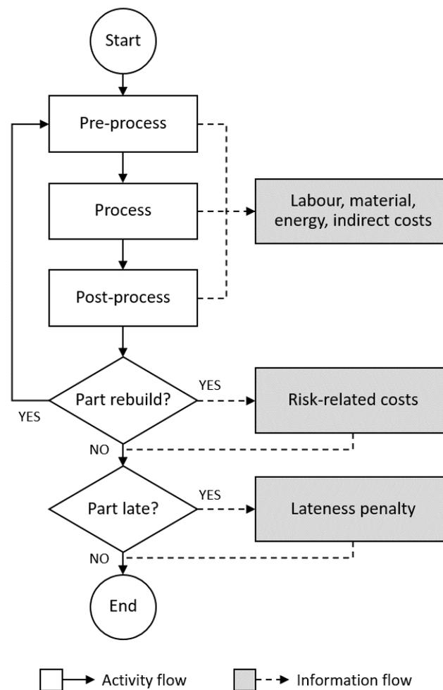
**Figure 3.13: AM process stages for polymer laser sintering and associated cost model elements**
