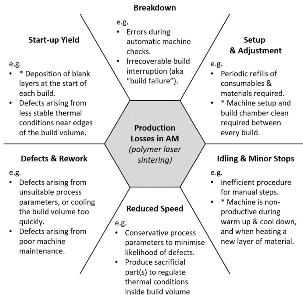
**Figure 4.2: Examples of production losses in polymer laser sintering workflow**
