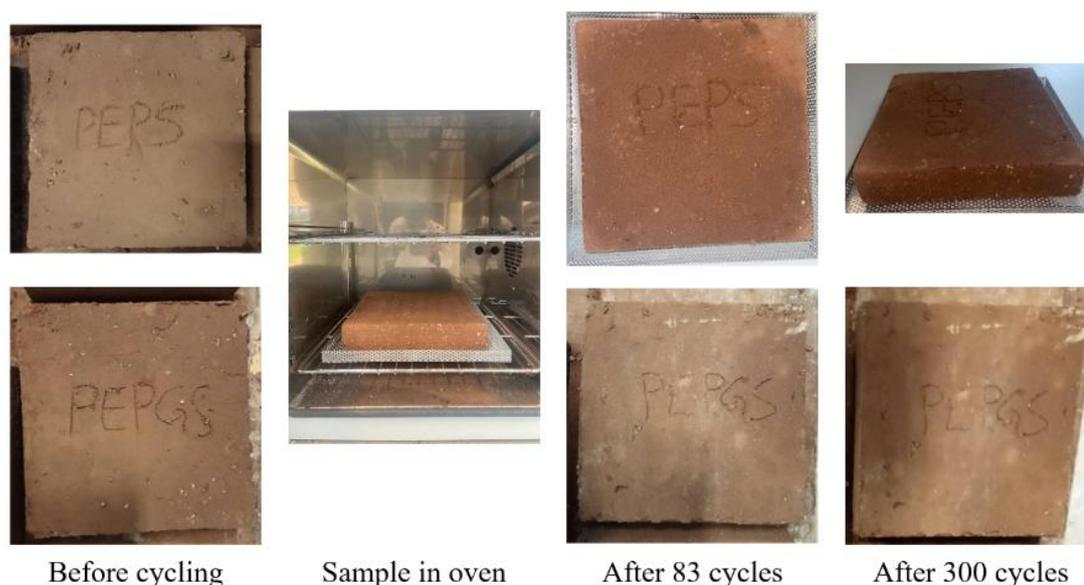
**Figure 3-7** Earthbag block thermal cycling process
