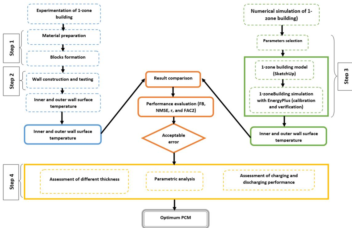
Figure 4-1 Flowchart of development of the earthbag-PCM model
