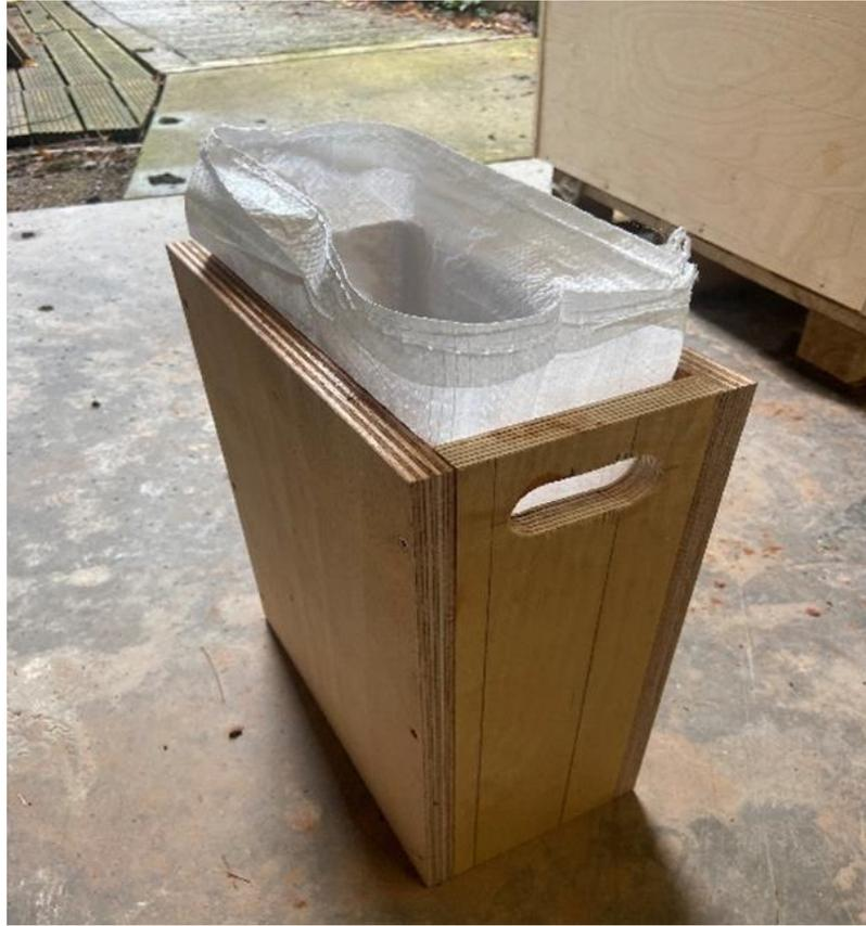
Figure 4-2 Earthbag block mould
