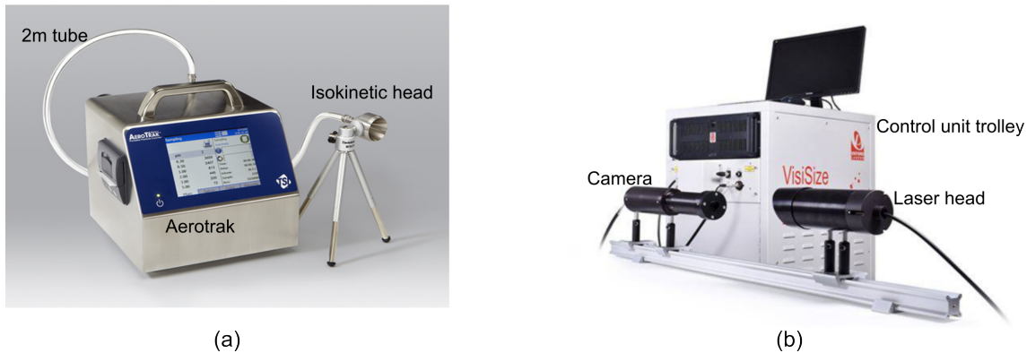
Figure 6.2: Instruments used for aerosol and droplet generation (a) Aerotrak [248] (b) VisiSize [249]
