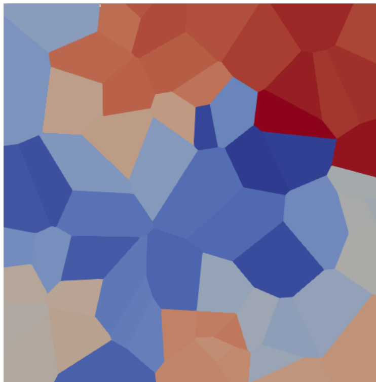
Figure 4.11: A Voronoi mesh with 64 elements.
