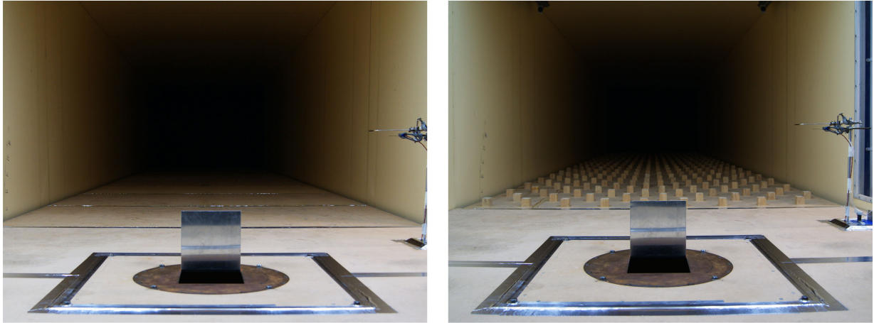
Figure 4.4: Alternative preconditioning elements used in the window characterisation experiments. The MDF sheets intended to create a thin boundary layer are shown on the left, and the roughness elements intended to create a thick boundary layer are shown on the right.
