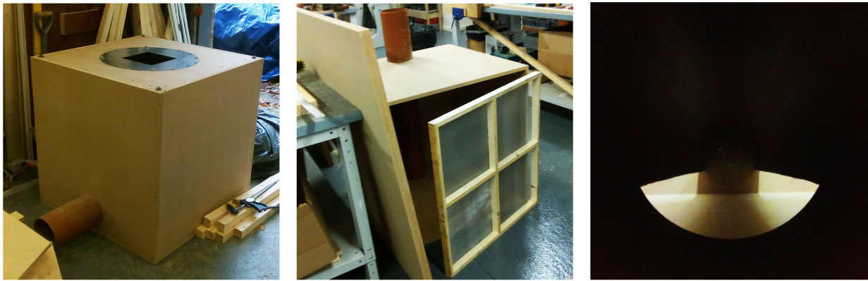
Figure 4.7: Plenum chamber (left) and details of the diffuser array (middle and right). The middle image depicts a partially constructed plenum, with the mesh filter visible. The right image depicts the interior of the supply duct, and the slits that distribute air into the plenum.
