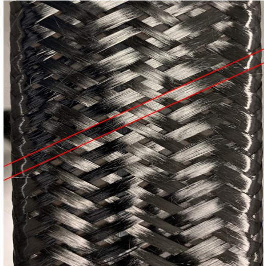
Figure A-6: Image of braid taken from square mandrel with yarn path highlighted in red.
