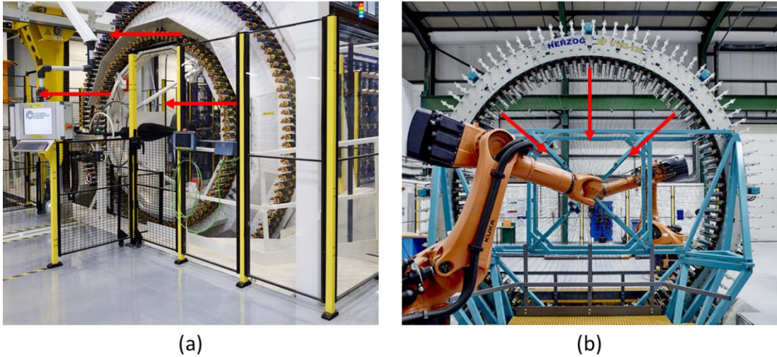
Figure 1-3. Examples of (a) axial braider and (b) radial braider with the direction of bobbins in respect to the spool plane shown by red arrows.
