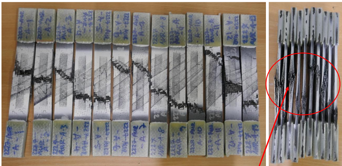
Evidence of delamination of layers
