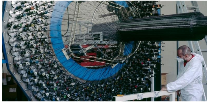
Figure 2-2. An example of a 3D braiding machine, the bobbins are able to move between multiple rings.
