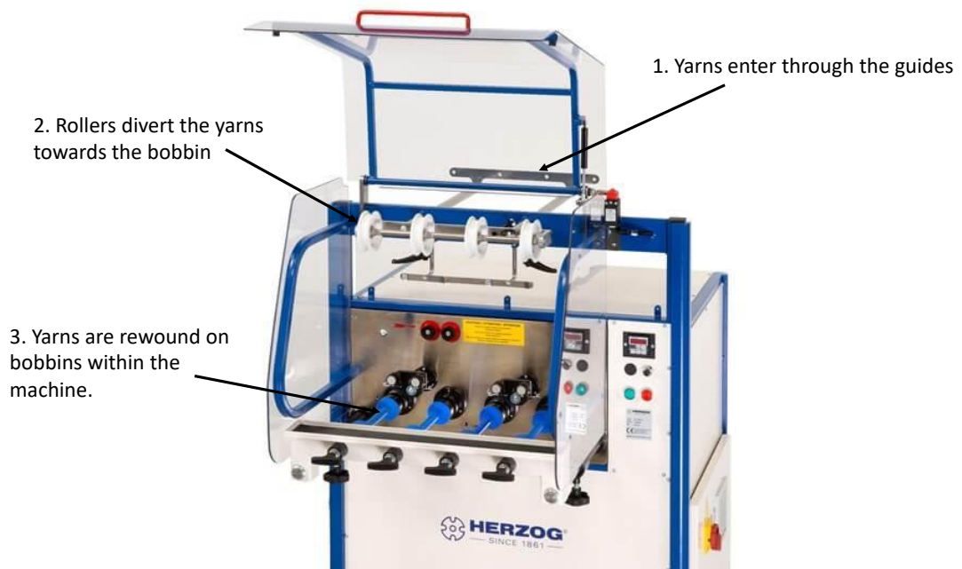
Figure 1-8: Herzog bobbin winding machine to wind yarns for braiding.[16]
