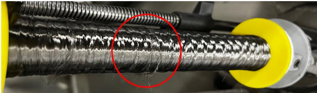
Figure 4-14. Fibrous ring observed during braiding on 0 tpm fibres causing yarn breakages.
