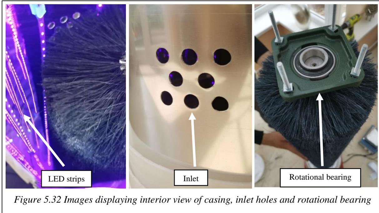
At the hub's summit, a wooden plate and bearing was used. The rotational bearing, as shown in Figure 5.32, would hold the hub in place but also allow it rotate smoothly. As this prototype would need to be dismantled so that the brush fibres could be changed for different testing criteria, the top of the prototype and casing could be removed easily to allow for this. The bearing was fixed to the lid and the prototype was complete.
