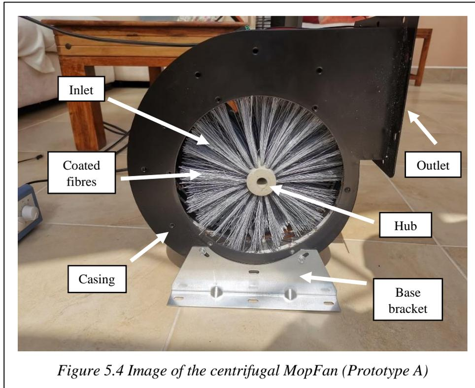
Figure 5.4 Image of the centrifugal MopFan (Prototype A)
