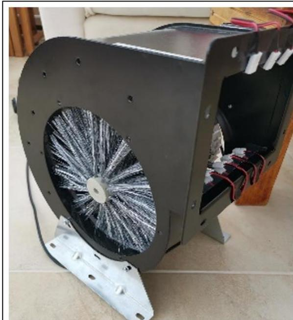
*Figure 6.7 Image of centrifugal fan
