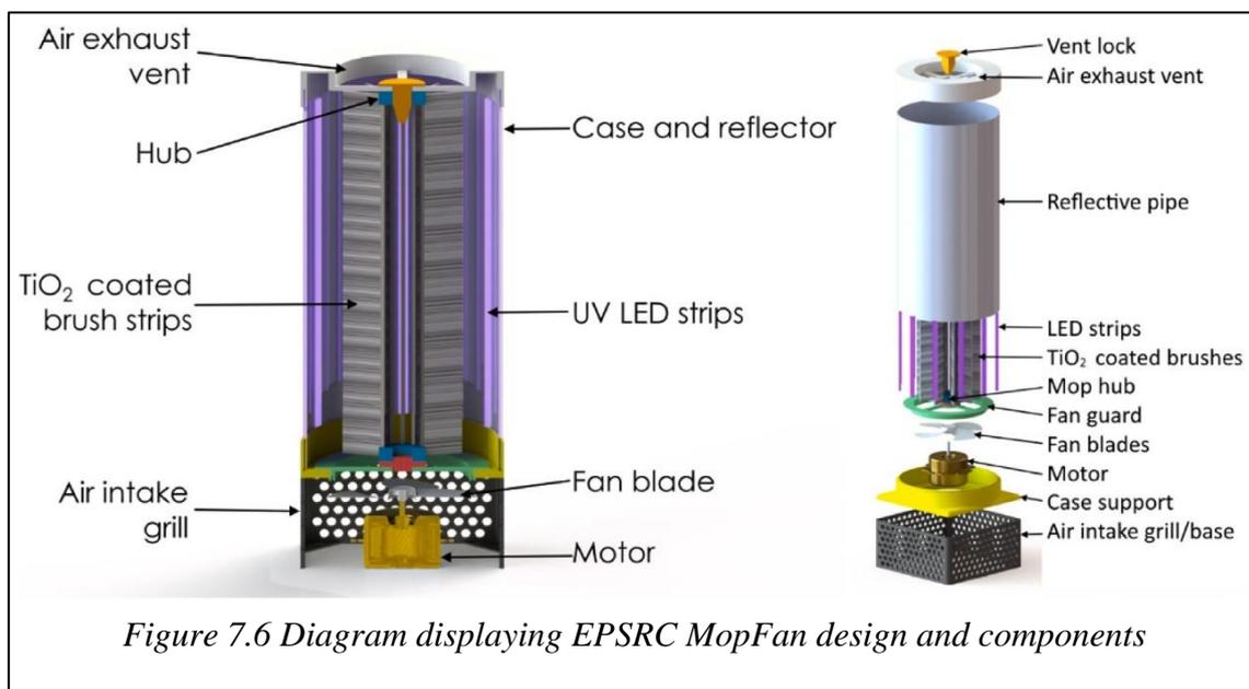
Figure 7.6 Diagram displaying EPSRC MopFan design and components
