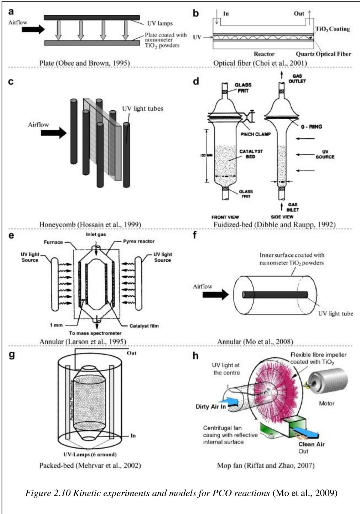
Figure 2.10 Kinetic experiments and models for PCO reactions (Mo et al., 2009)
