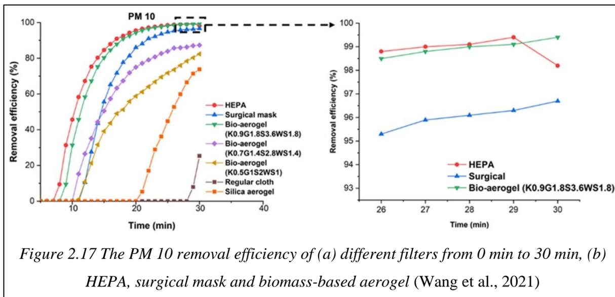
Figure 2.17 The PM 10 removal efficiency of (a) different filters from 0 min to 30 min, (b) HEPA, surgical mask and biomass-based aerogel (Wang et al., 2021)
