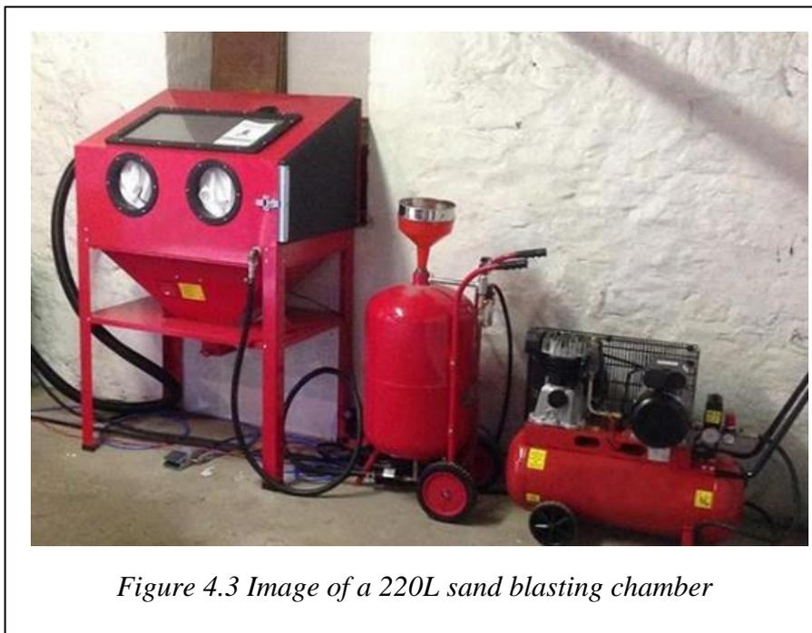
*Figure 4.3 Image of a 220L sand blasting chamber*
