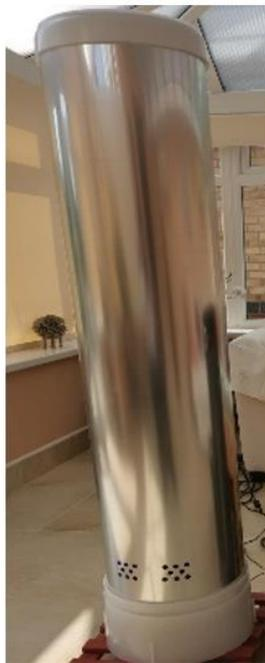
*Figure 6.17 Large-scale tower fan prior to testing (Prototype C)*
