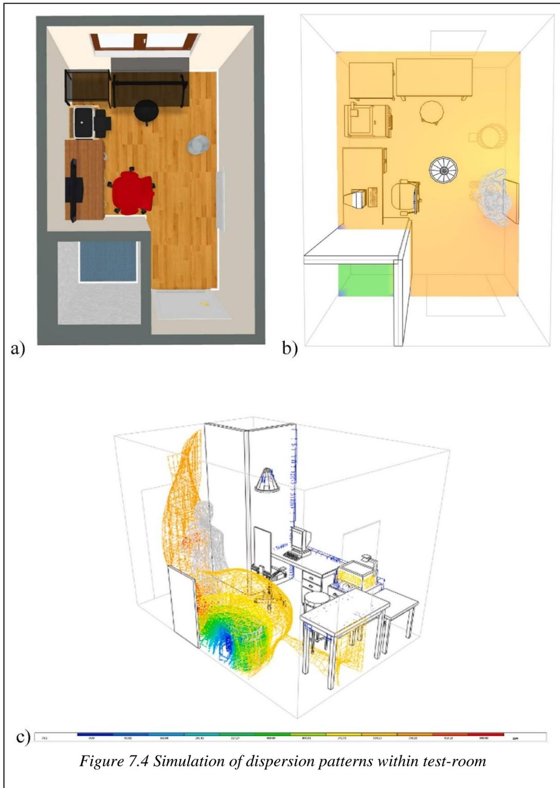
Figure 7.4 Simulation of dispersion patterns within test-room
