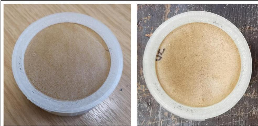
*Figure A.3 Bio-aerogel filter before and after particle testing*
