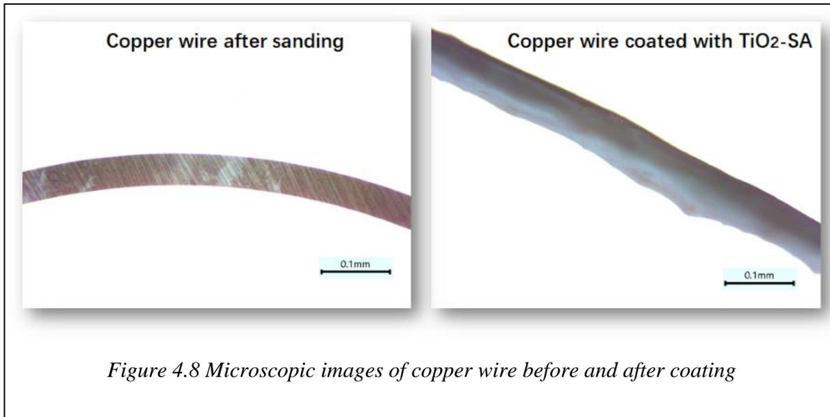
*Figure 4.8 Microscopic images of copper wire before and after coating*
