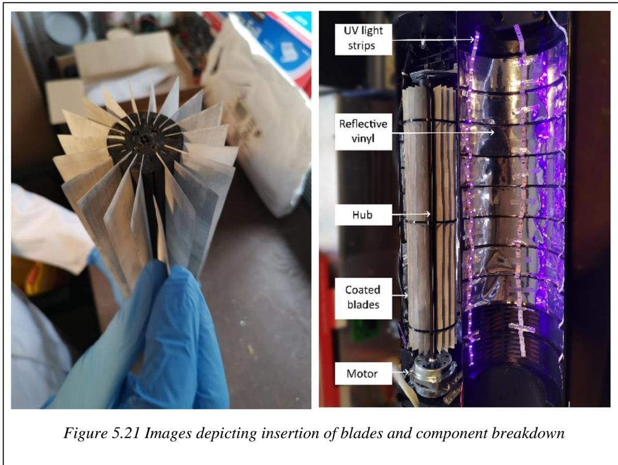
Figure 5.21 Images depicting insertion of blades and component breakdown
