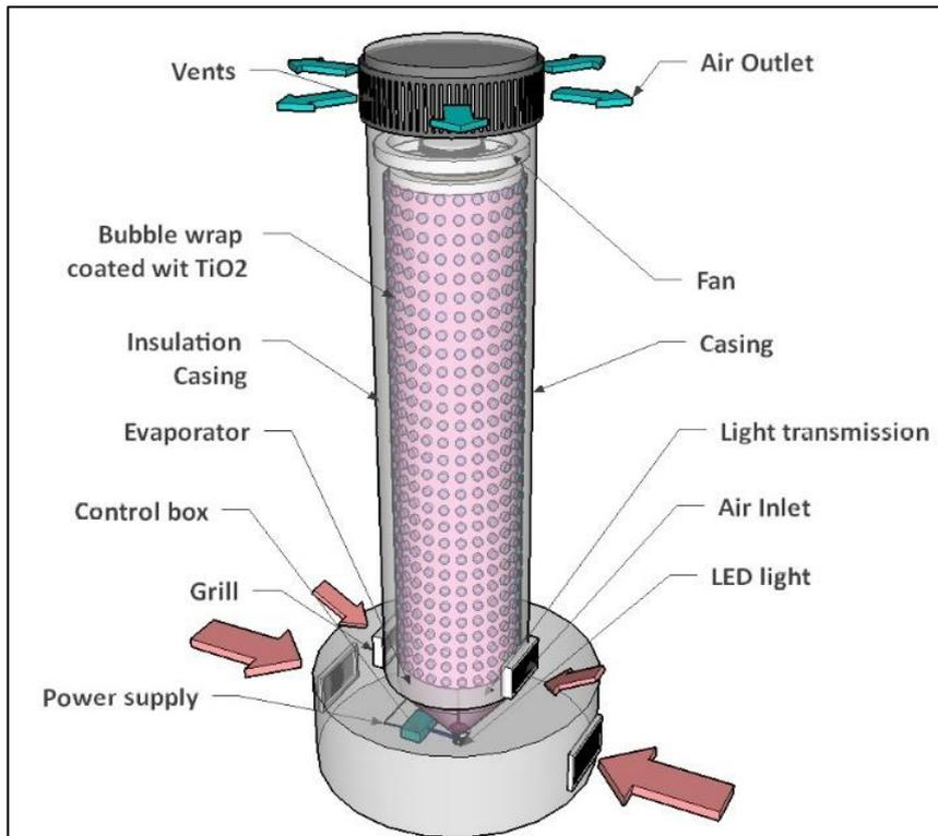
Figure A.10 Diagram of MopFan prototype using  $\text{TiO}_2$  coated bubble wrap
