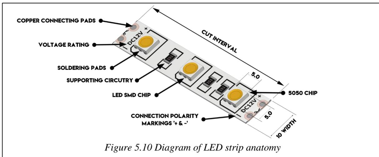
Figure 5.10 Diagram of LED strip anatomy
