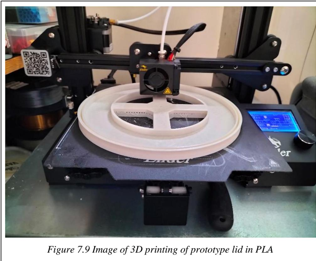
*Figure 7.9 Image of 3D printing of prototype lid in PLA*
