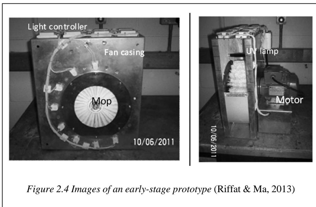
Figure 2.4 Images of an early-stage prototype (Riffat & Ma, 2013)
