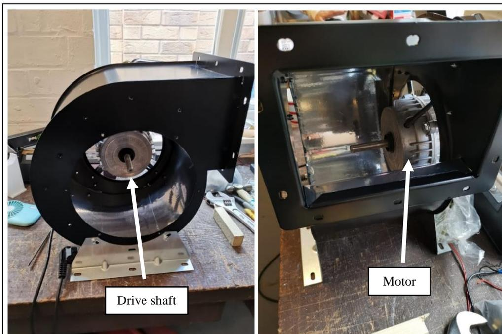
*Figure 5.11 Images of a dismantled centrifugal fan*
