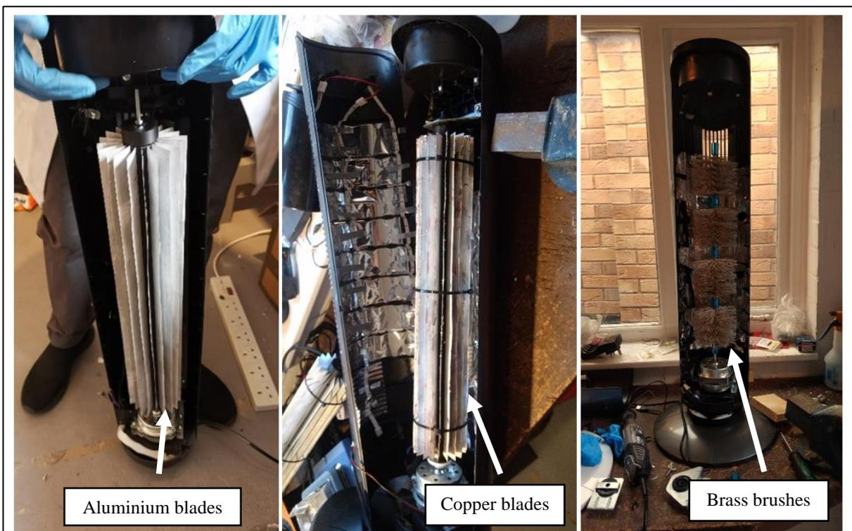
*Figure 5.20 Images of alternative hubs (Aluminium, copper and brass brush)*
