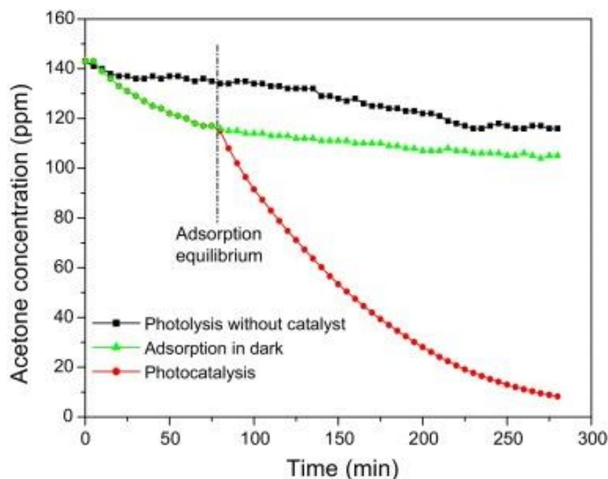
Figure 2.6 Graph displaying acetone concentration tests using photocatalysis (Pétigny et al., 2021)
