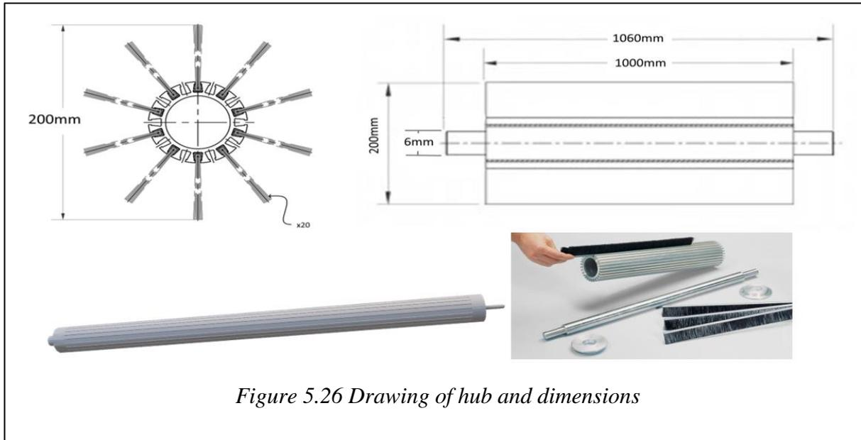
*Figure 5.26 Drawing of hub and dimensions*
