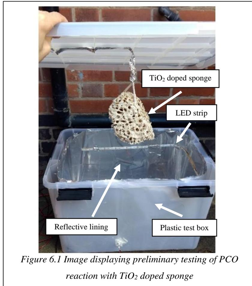
*Figure 6.1 Image displaying preliminary testing of PCO reaction with TiO<sub>2</sub> doped sponge*
