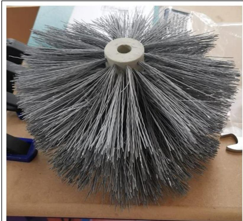
*Figure 5.8 Image of the custom-made impeller for Prototype A*
