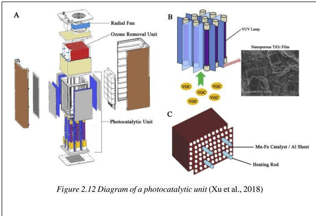
Figure 2.12 Diagram of a photocatalytic unit (Xu et al., 2018)
