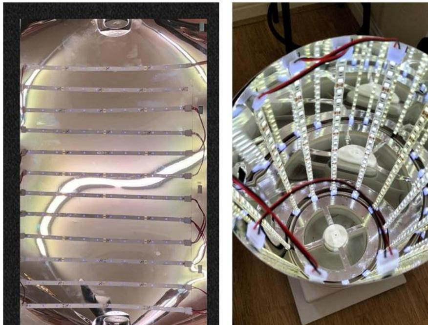
*Figure A.9 Image of LED distribution within UV enhanced aluminium casing*
