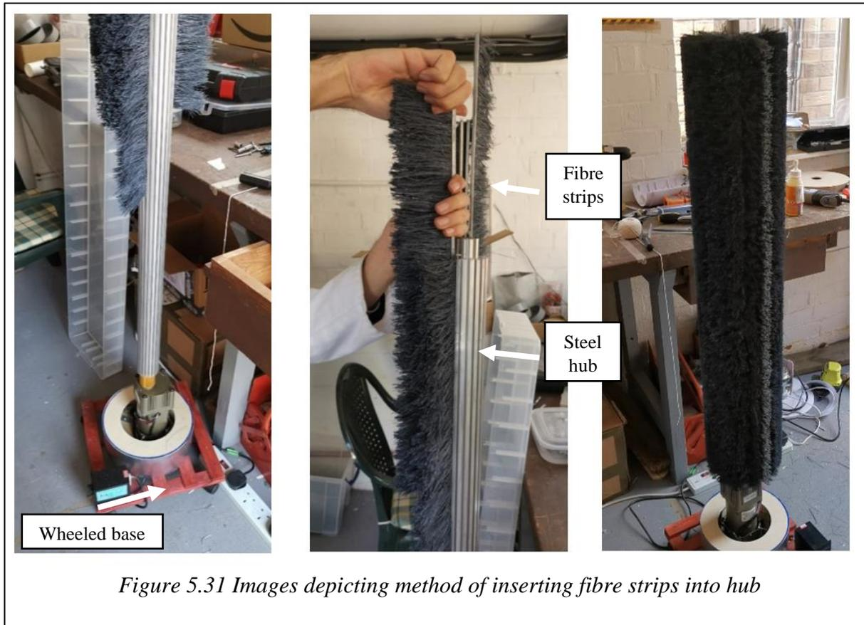
*Figure 5.31 Images depicting method of inserting fibre strips into hub*
