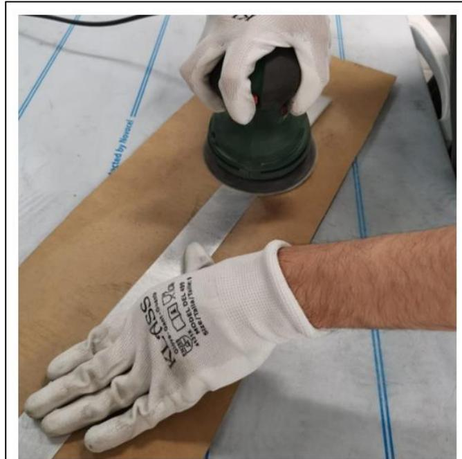
*Figure 5.18 Image of rotary sanding of aluminium strip in preparation for coating*
