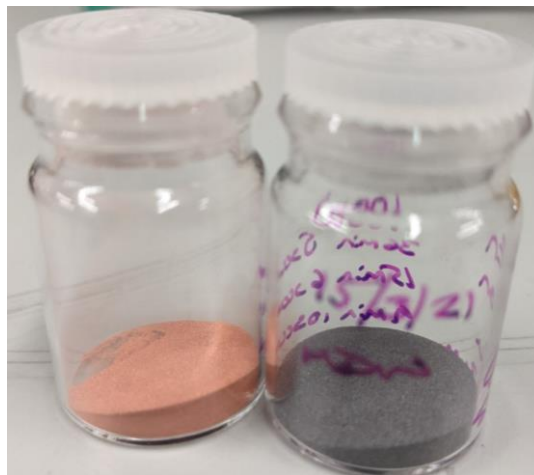
Figure 34 - Photo of two powders in glass vials, left) uncoated Cu-Coarse, right) Cu-Zn-Coarse coated with Zn, with distinct change in colour.
