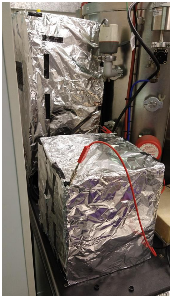
Figure 106 - Photo of the mesh/foil Faraday cages in place covering Mag 4 (far) and the gas mass flow controllers (MFCs) (near).
