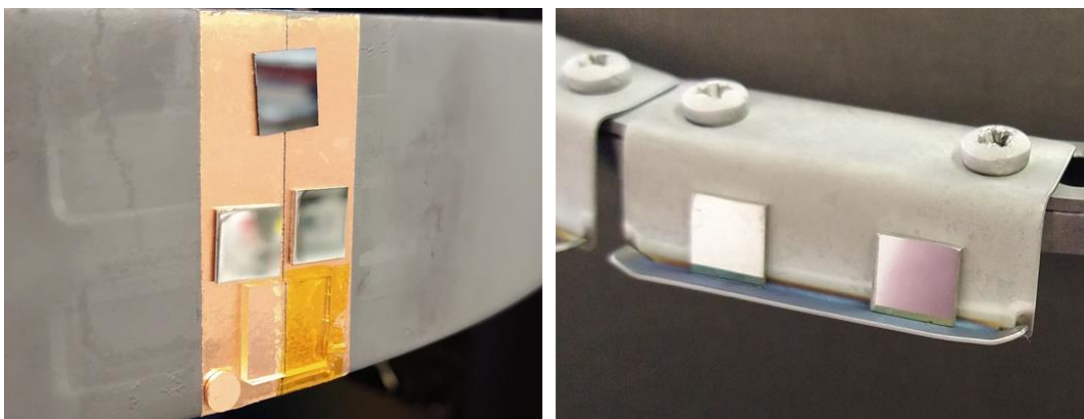
Figure 24 - Photos of the two different arrangements of substrates on the holder, substrates are uncoated, a) stuck to the holder using double side adhesive copper tape, materials from top to bottom, silicon, steel, glass b) resting on bent stainless steel ledges, 2 steel coupons.
