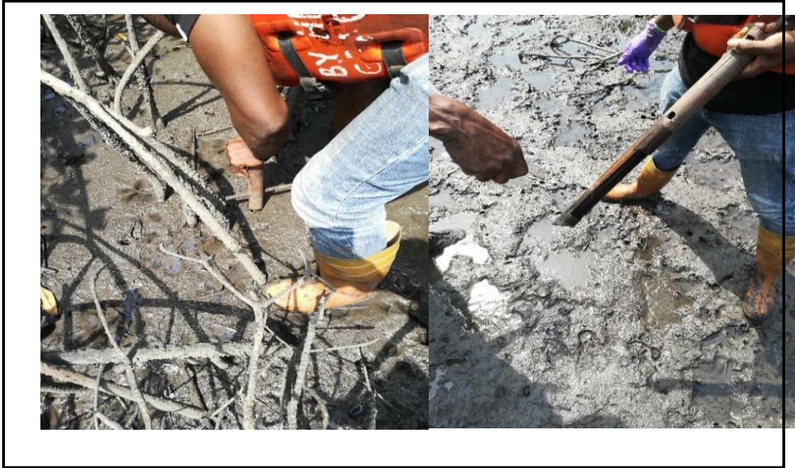
Figure 5.5: Soil samples were taken with a portable auger.
