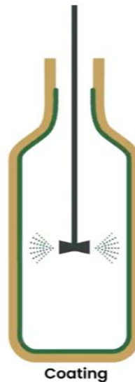
Figure 9: Image of spray coating technique used by Pulpex to produce an inner protective coating of the bottle. Source: (Pulpex, 2022)
