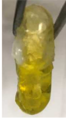
Figure 2.3. Cracking of the pre-assembled and pre-filled HPMC capsule upon dip-coating.
