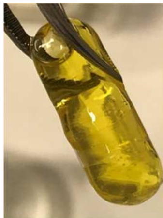
Figure 2.4. Pre-filled HPMC capsule dip-coated into the Eudragit® S and TEC solution.
