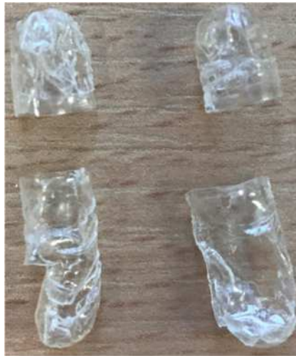
Figure 2.2. Brittles and cracks on the HPMC capsule shells upon dip-coating in the 16.7% Eudragit® S 100 solution.
