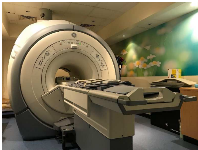
Figure 5.4. The 1.5T XDxt MRI scanner at the Sir Peter Mansfield Imaging Centre at the University of Nottingham. The full body coil used for this study is visible on the scanner bed.
