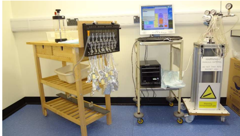
Figure 5.3. The MRI compatible, 16 channel perfused manometry system used in this study is shown on the left. The computer and medical air pressure cylinder shown on the right remained in the scanner control room with cables and tubing to the MRI-compatible system in the scanner room passed through a wave guide in the wall.
