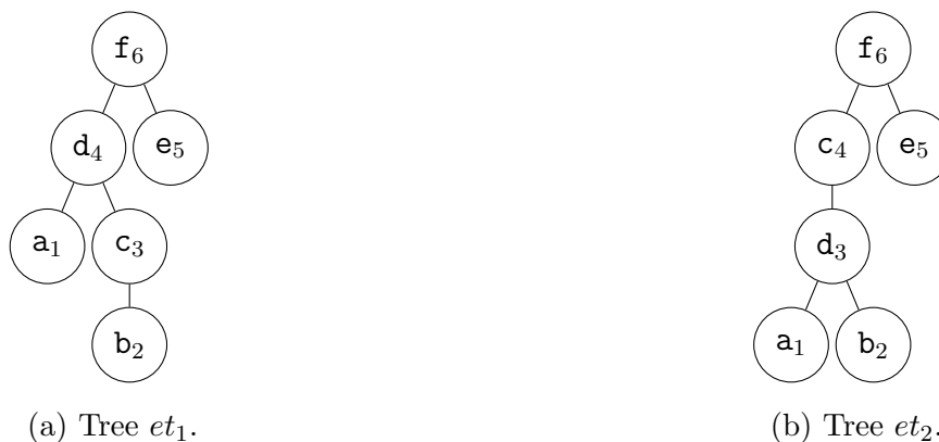
Figure 2.14: Two trees that are used in Section 2.6.2 to illustrate how the MTED algorithm works. In each node in each tree we mark the index according to a post-order traversal.
