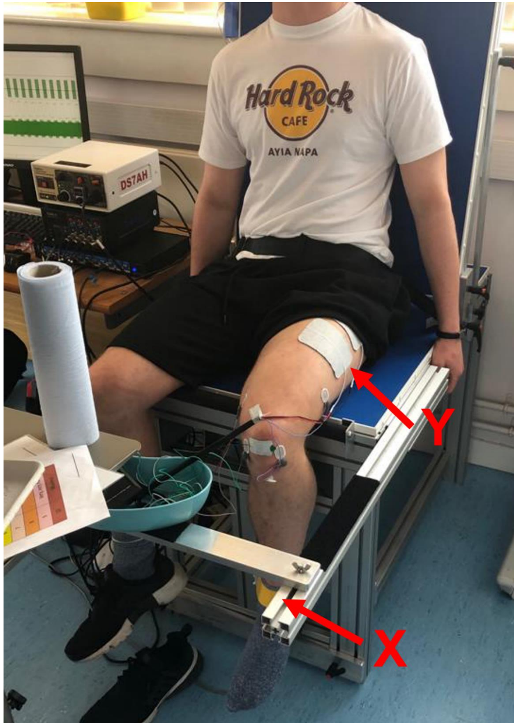
Figure 6.1: A picture showing the custom dynamometer 'Derby Chair' with the participant's knee joint fixed at 90 degrees with an ankle strap (X) to perform maximal voluntary isometric contractions against a force transducer. Also shown are the stimulation electrodes in position for NMES (Y).
