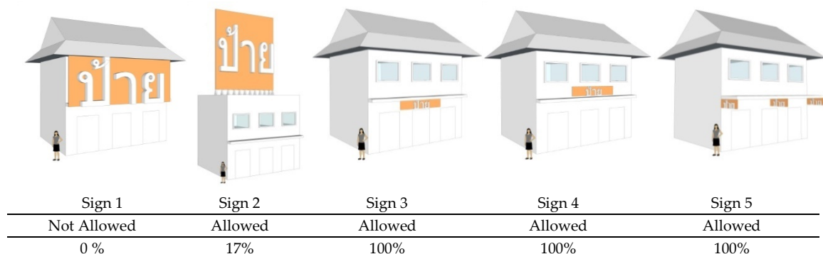
Figure 7-17: The simulation of commercial signs allowance in Chiang Mai Municipal building Law (Author)
