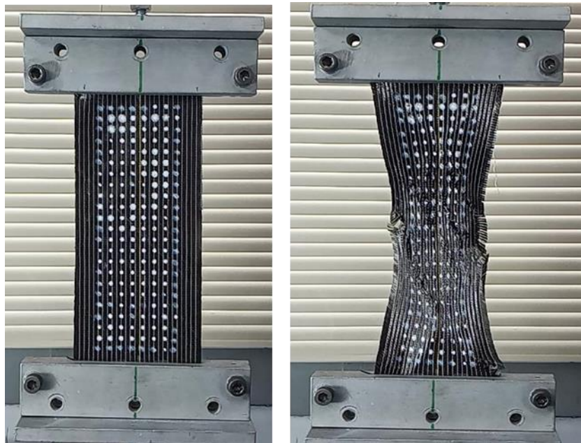
Figure 5-1 Comparison of the sample shape during the bias extension test of FCIM789 before cycle 1(a) and during cycle 1(b).
