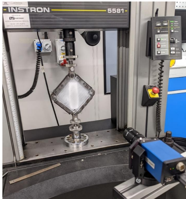
Figure 4-6 Yarn slippage video gauge measurement (Keyence CV-X Series) setup for in-plane shear testing
