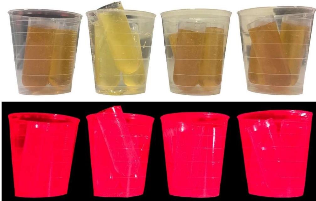
Figure 2-2. Using red light to minimise the colour difference among model foods. Top: before applying the red light, bottom: after applying the red light.
