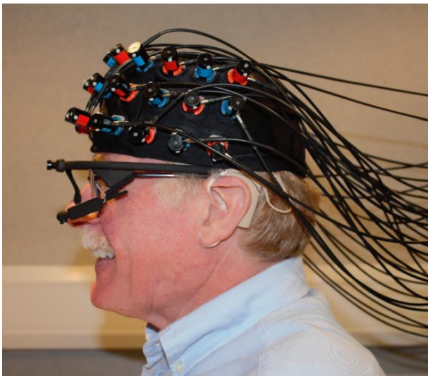
Figure 3.1. Typical placement of the Pupil Labs eye-tracker and the fNIRS headset (optode array: 3x11) over participants’ head. Photograph of typical equipment setup on a volunteer’s head.
