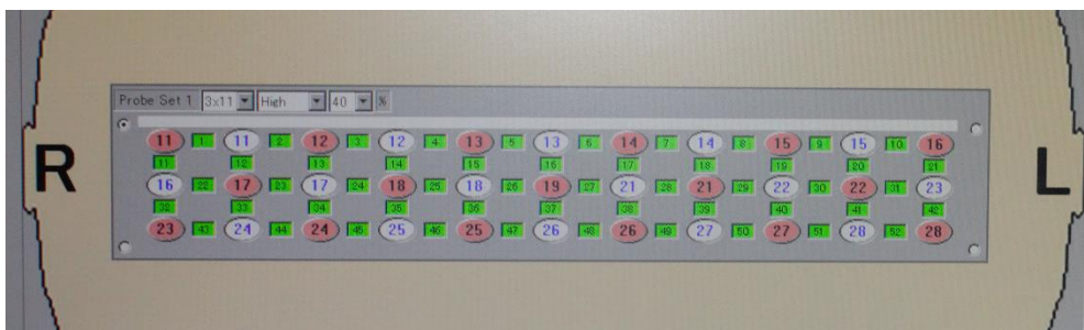
Figure 3.2. An example of the optode-scalp contact profile provided by the Auto Gain feature of the Hitachi ETG-4000 fNIRS system. The example shown displays an optimal optode-scalp contact as indicated by the green channels.
